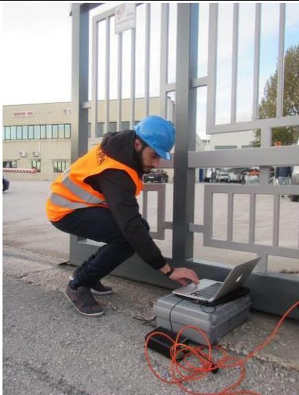
**Misura trasversale allineamento vibratori: 10 m - ASFALTO**
