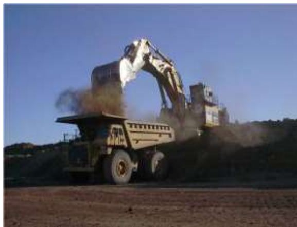
Figura 53 Truck Loading: Overburden SCC 05-010-37
