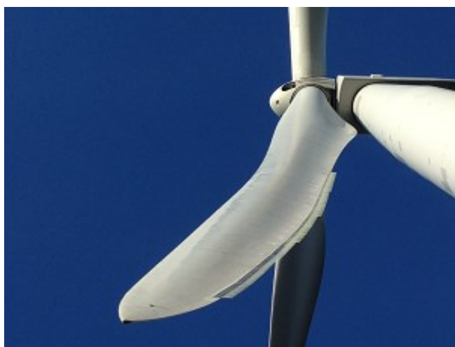
Fig. 1: LNTes at the wind turbine rotor blade
