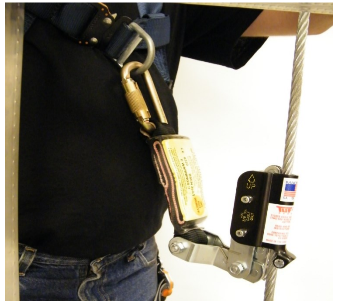
Fig. 6: Usage of the wire grab fall arrestor (example)
