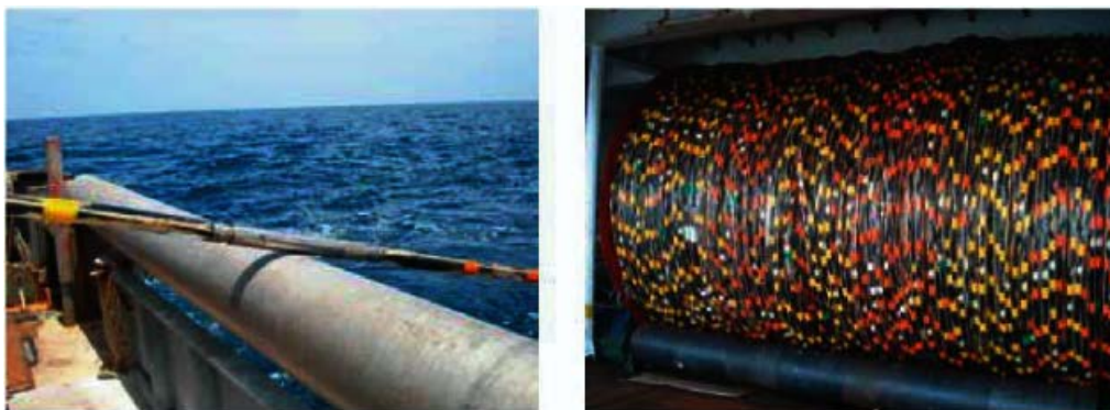
FIGURE 2.19: PATTERN OF SEISMIC CABLE OR STREAMER (OGP, 2011)
