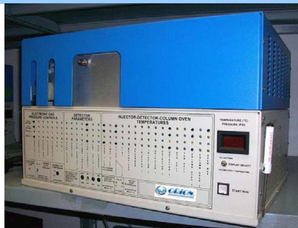
**Orion BTX-2000** is an SRI gas-chromatograph analyser specifically configured for the analysis of BTX (benzene, toluene, o-xylene). The working principle is based on pre-concentrating the analytes into an adsorbing trap material and then make the gas chromatographic analysis using a photo-ionization detector.
