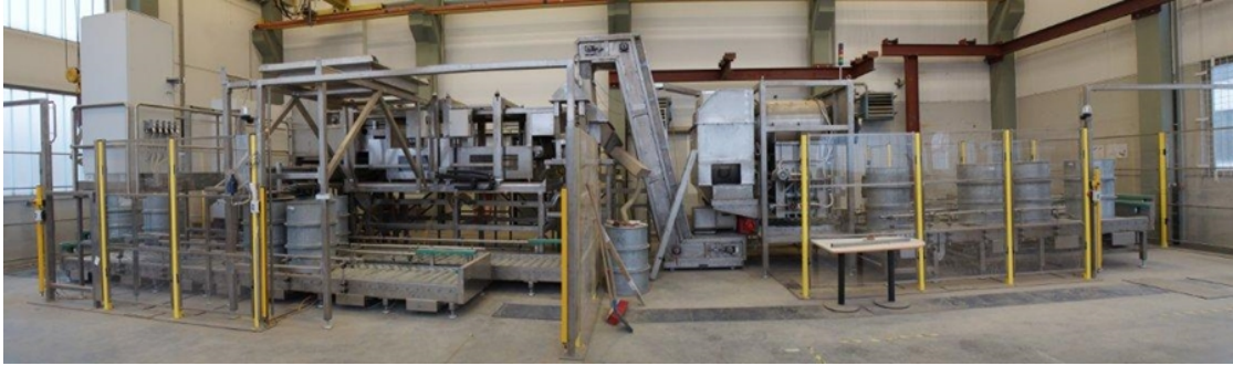
Figure 7: Soil measuring system (right material application, left measurement and separation)
