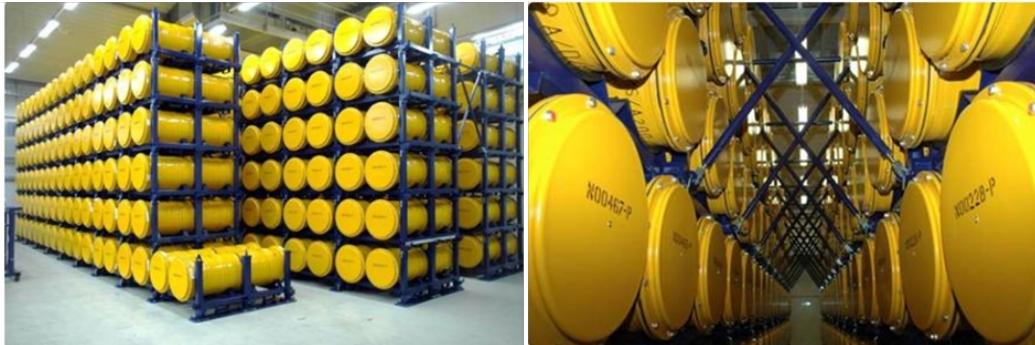
Figure 5: Interim storage of the conditioned 200 litre drums
