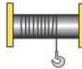
WL-800 m (B) drum capacity of 5 mm wire diameter (2 600 ft of 0.19 in) with a wire levelling device, mounted underneath the feed frame.
