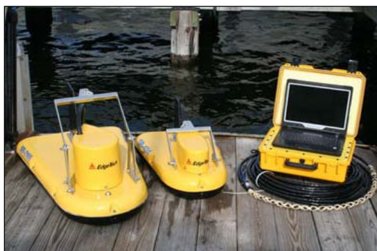
Fig. 7 - Hardware e Towfish SBP Edge Tech 3100P
