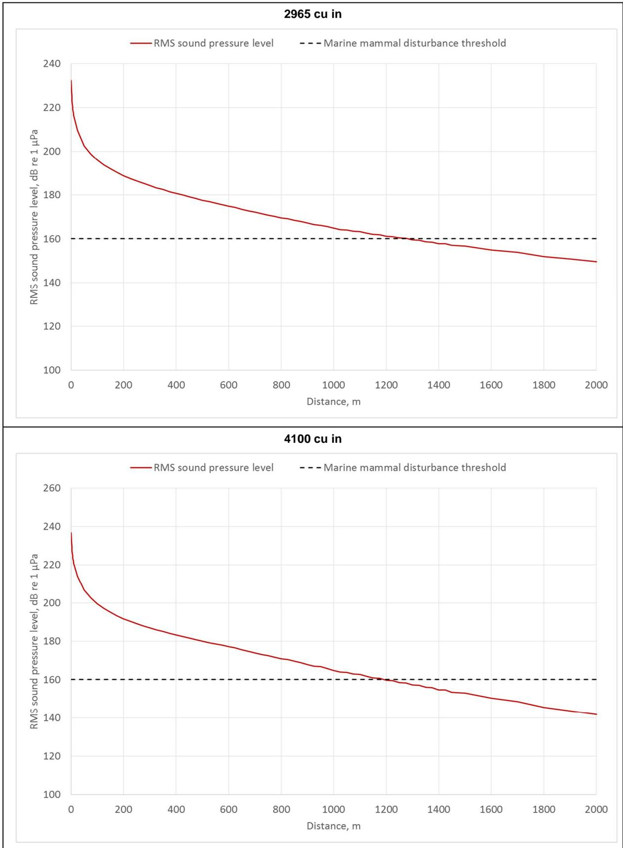
Figure 5.3  $RMS_{T90}$  sound pressure level against distance for behavioural change
