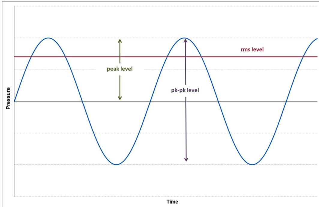
**Figure 2.1 Graphical representation of acoustic wave descriptors**
