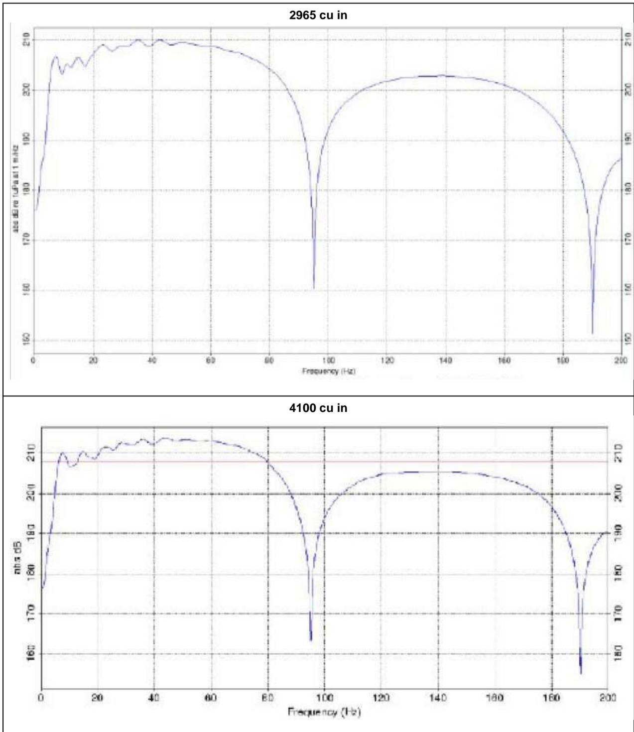
**Figure 4.2 Source frequency characteristics (250 Hz low-pass filtered)**
