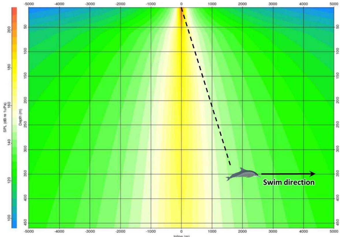
**Figure 4.4 Example inline SPL showing array directivity**
