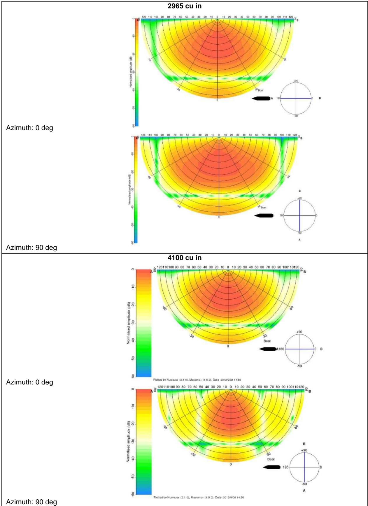
**Figure 4.3** Directivity plots for source array
