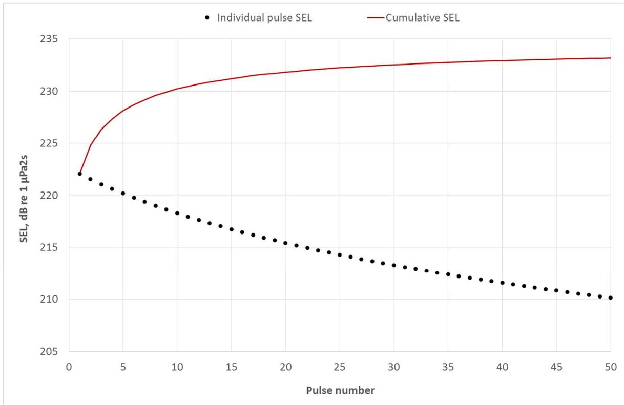
**Figure 4.10 Discrete pulse SEL and cumulative SEL**
