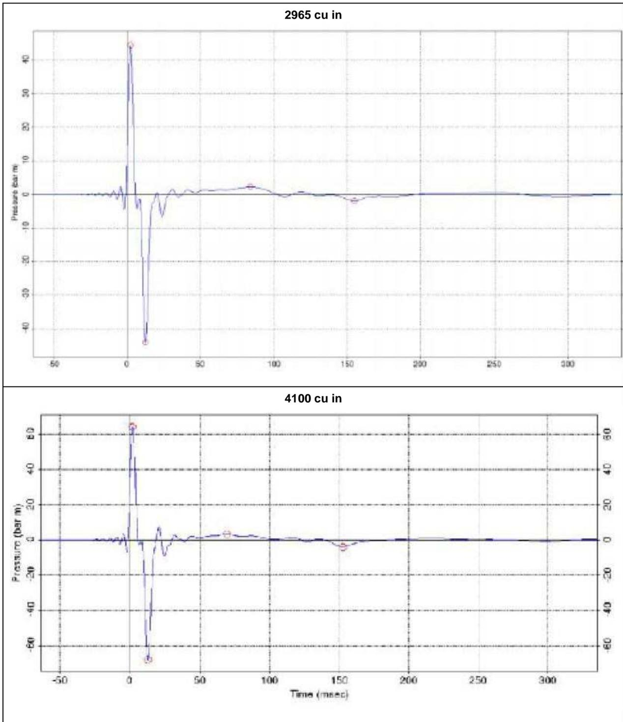
**Figure 4.1 Airgun array source time signature**
