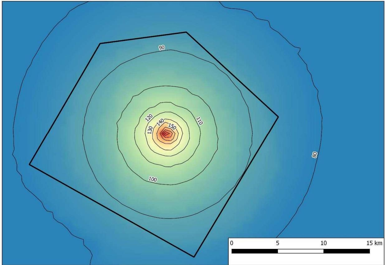
**Figure 5.4** **RMS<sub>T90</sub> sound pressure level contour, dB re 1 µPa (rms)**
