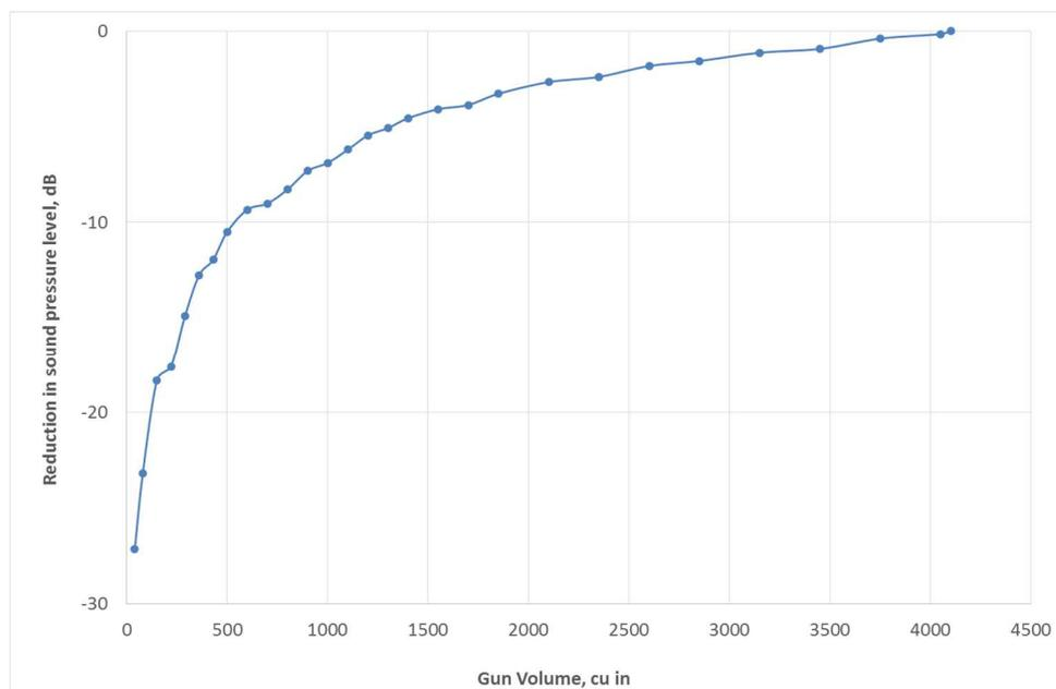
**Figure 4.11 Gun volume vs reduction in sound pressure level**
