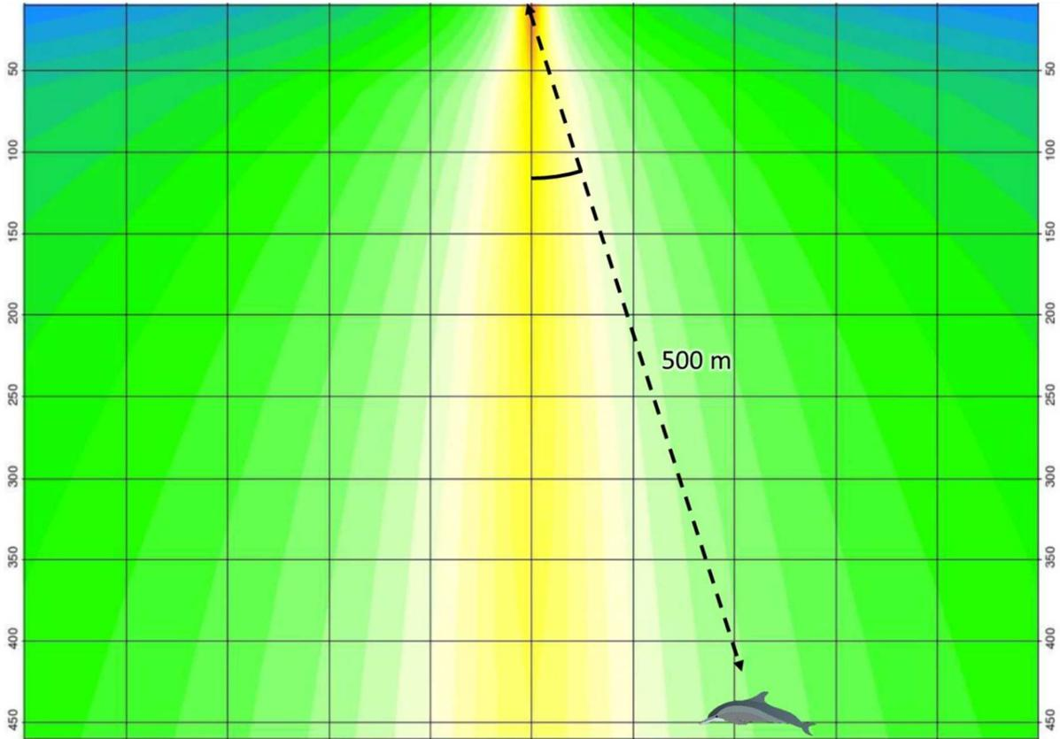
**Figure 4.6** Example showing injury range slightly larger than water depth
