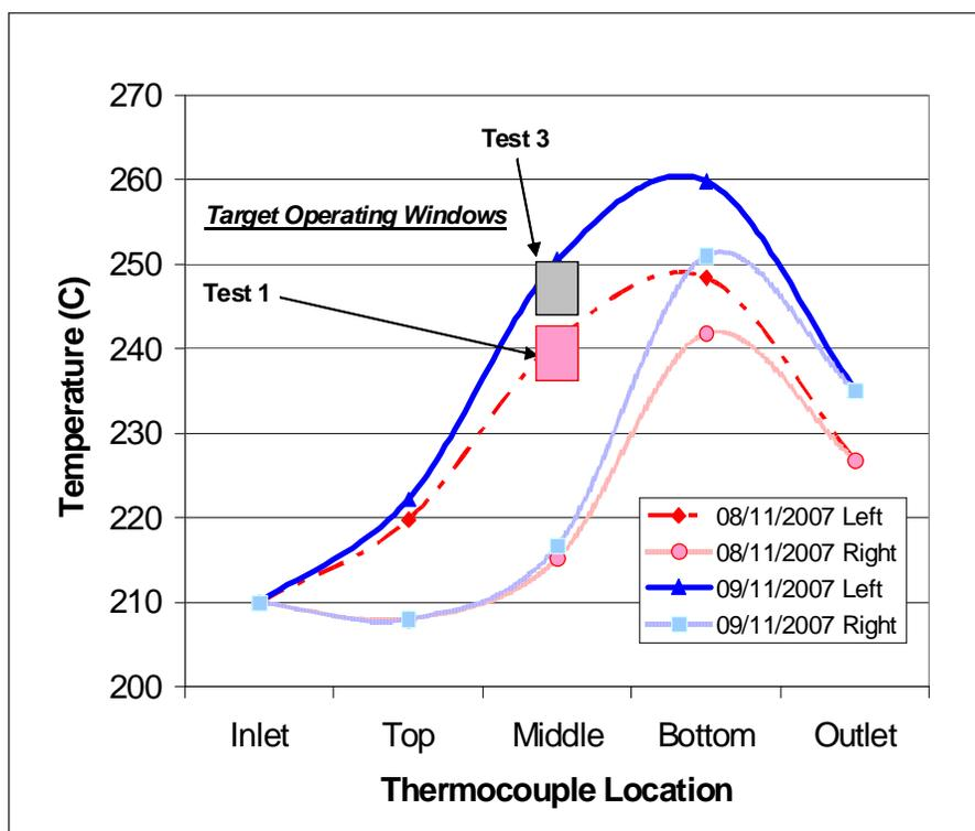
Figure 2.2-3 - SuperClaus Temperature Profile
