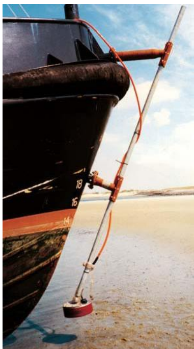
A single Sonar Head mounted at the bow of a small vessel.
