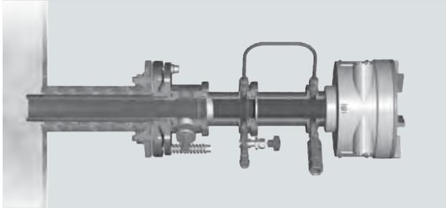
Sensor configuration with high purging on process side, with 6 mm joint for use with steam, and with N<sub>2</sub> purging on the sensor side
