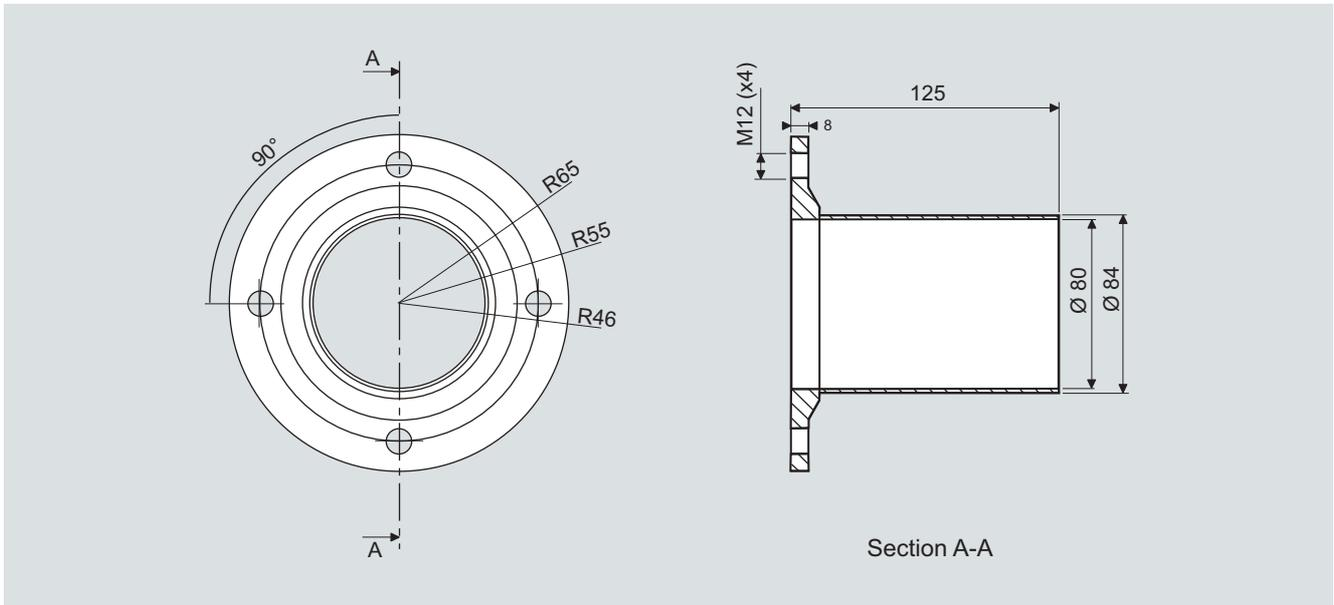
Weld-on flange, sensor option, dimensions in mm
