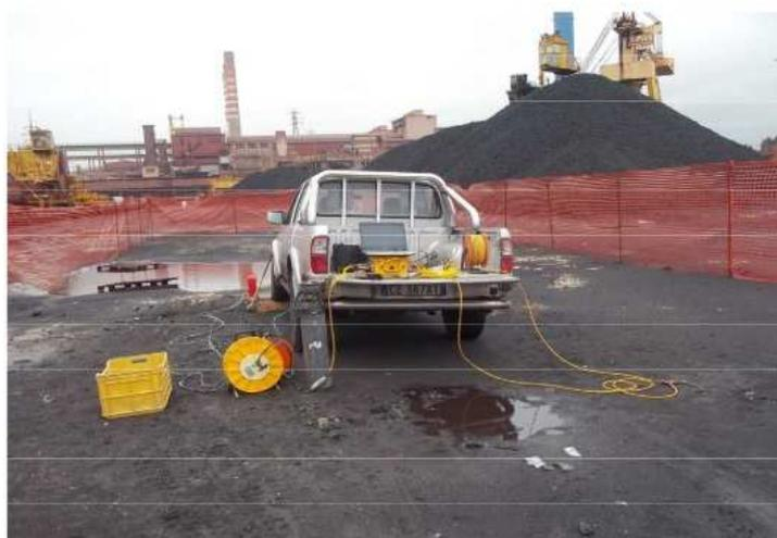
Fig. 2.2.4.3 Rilievo sismico in foro Down- hole – Parco omo
