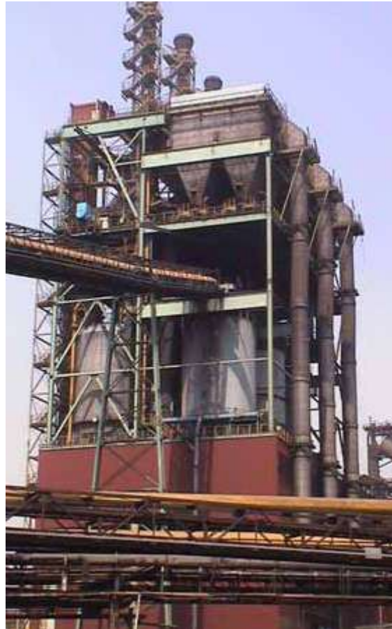
Sistema P.C.I.(Powdered Coal Injection)
