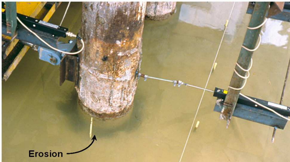
Figure 3-16 Annular Gapping Developed Around Pile After Cyclic Loading
