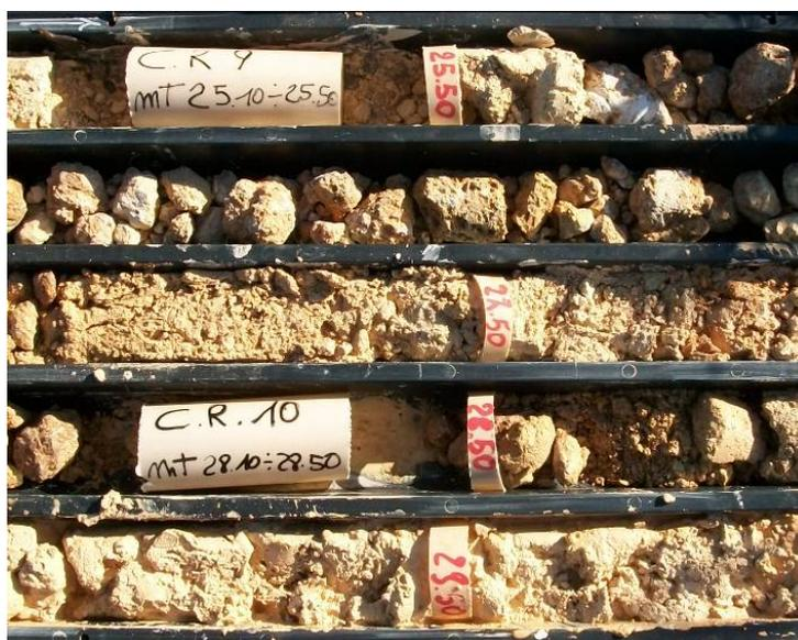
Fig 29 - Facies in sondaggio del Calcare Cavernoso (Cv) (Sondaggi 3/1-SD5, 3/1-SD4, 3/1-sd3)
