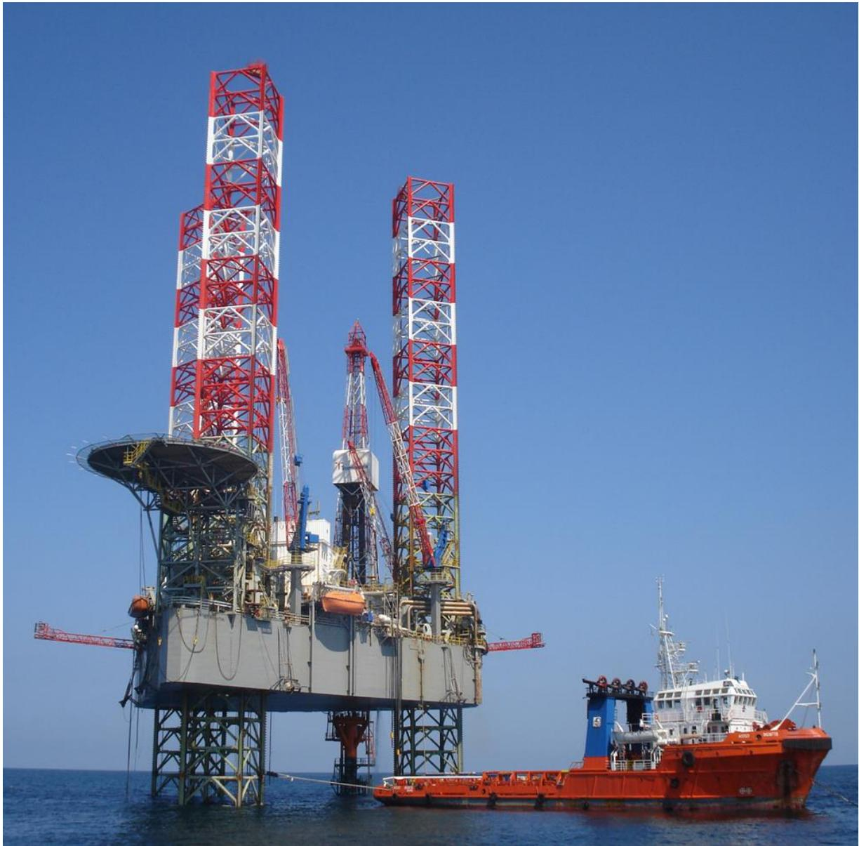
**Figura 3-7: Impianto Jack – Up Drilling Unit (tipo “GSF Key Manhattan”)**
