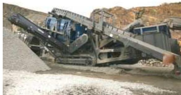
Secondary crushing mobile SCC 3-05-020-02
