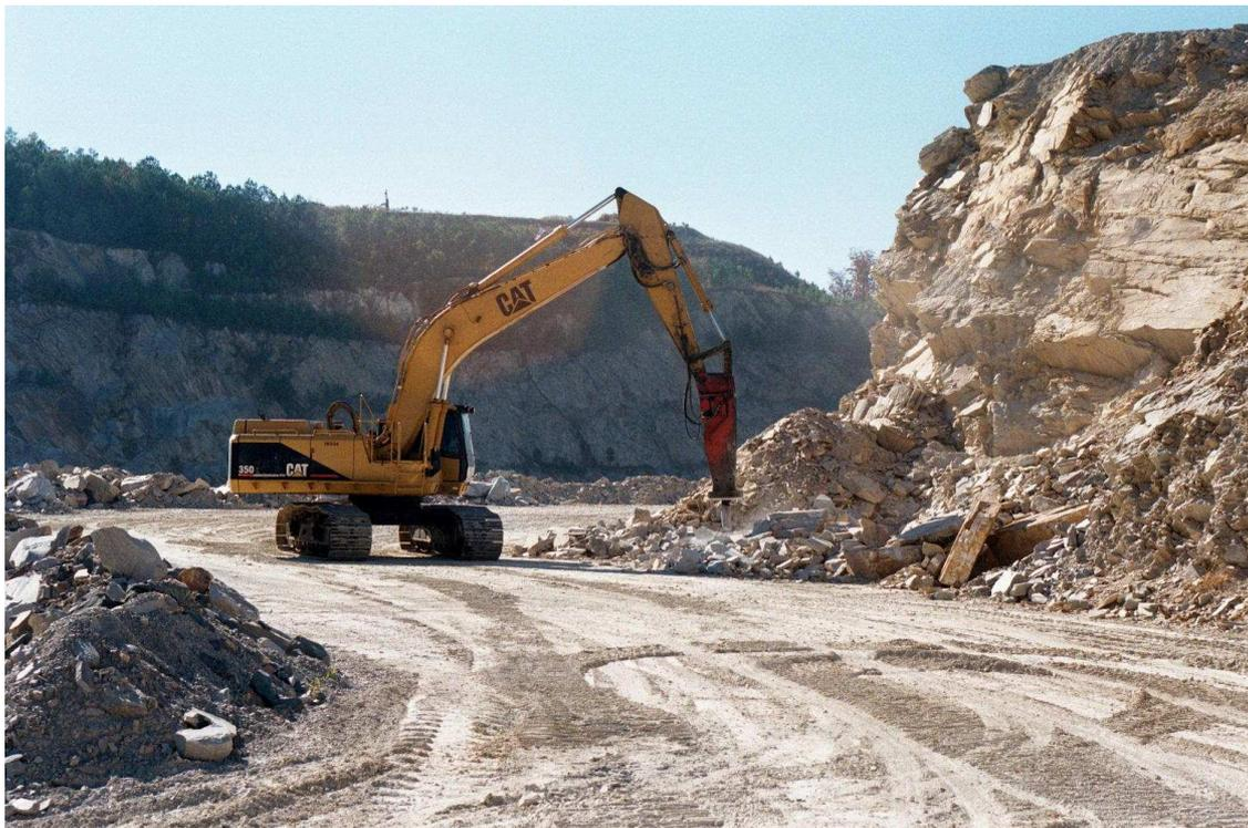
Primary Crushing (blast over size reduce) SCC 3-05-020-01
