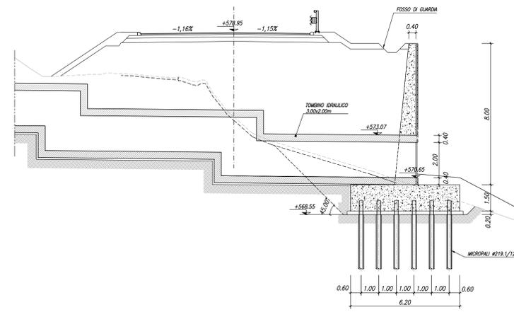
MURO TIPO "A" (H = >6-8m) - CARPENTERIA
