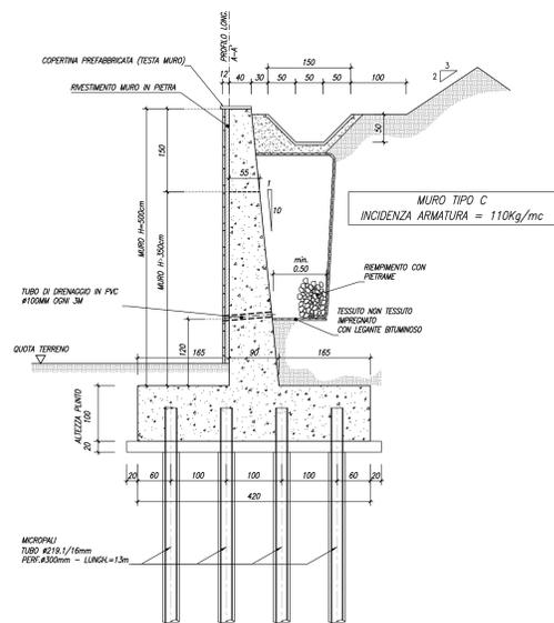
MURO TIPO "D" (H = >3.5-5m) - CARPENTERIA
