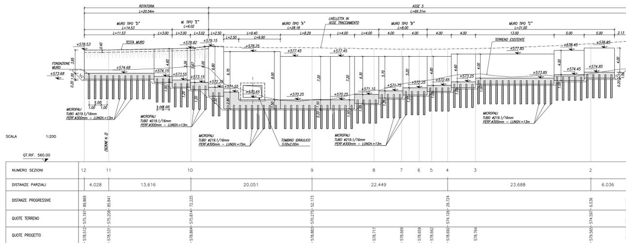
COLLEGAMENTO TOMBINO IDRAULICO-MURO CARPENTERIA
