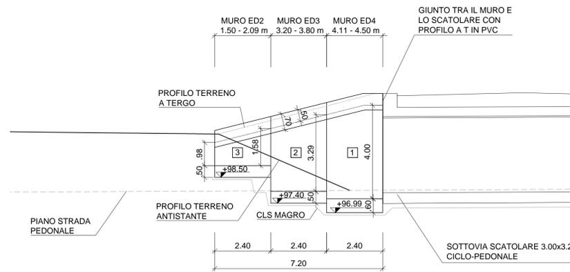
PIANTA MURO NORD-EST - SCALA 1:100
