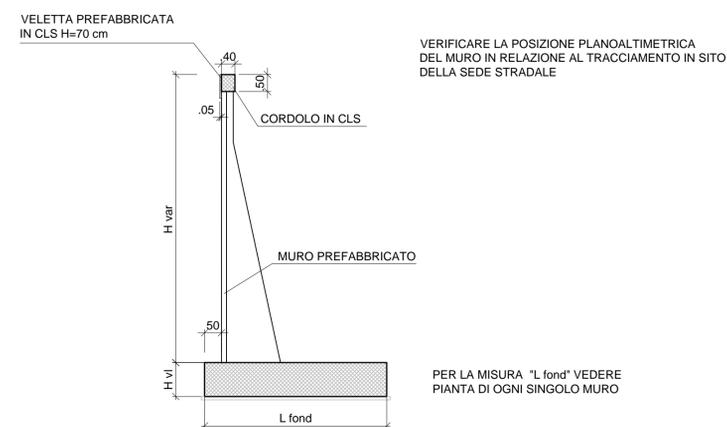
PROSPETTO A-A MURO NORD-EST - SCALA 1:100
