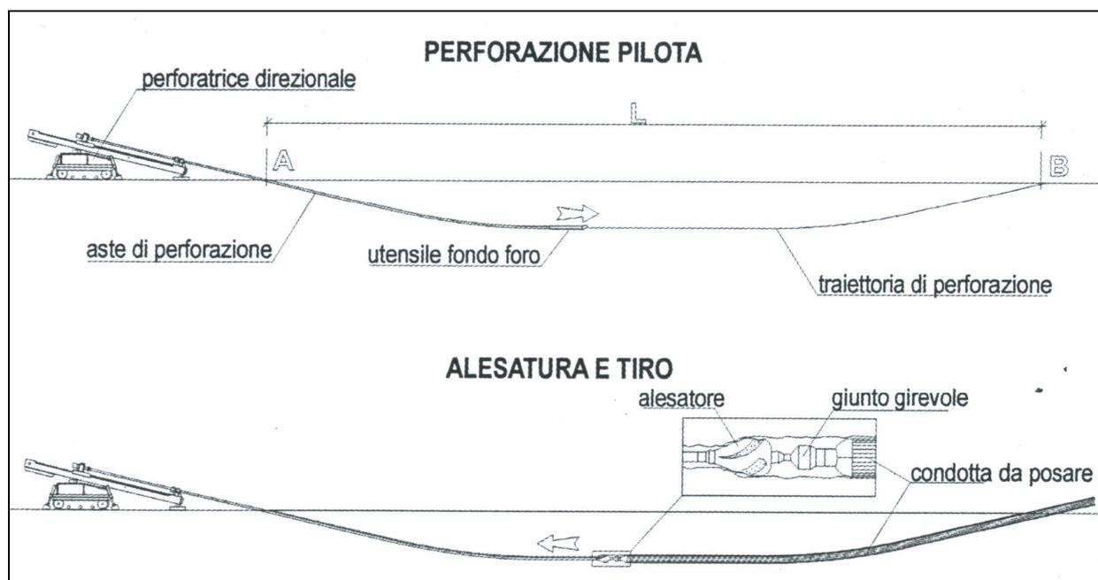
**Fig. 2** - Directional drilling
