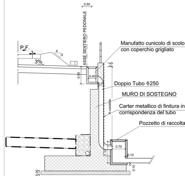
COLLETTORE DI SCARICO DA CANALETTA IN TESTA MURO CON B.A.
