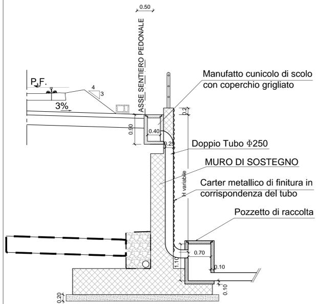
COLLETORE DI SCARICO DA CANALETTA IN TESTA MURO CON B.A.
