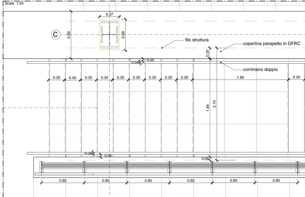
RIVESTIMENTO PILASTRO BANCHINA CENTRALE (D16)
