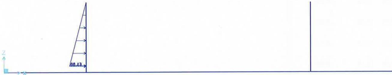
**FIGURA 8-3: DIAGRAMMA DELLA SPINTA A RIPOSO DOVUTA AL TERRENO A TERGO DEL MURO**
