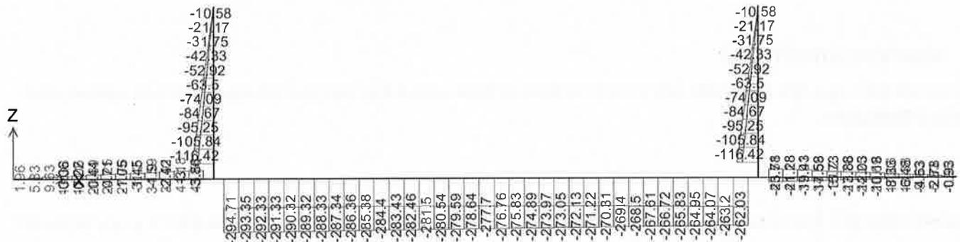
**FIGURA 8-15: SFORZO NORMALE - INVOLUPPO SLU/SLV**
