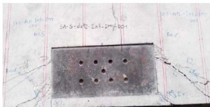
Figure 11: Typical failure mode obtained for 4x2 groups
