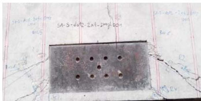
**Figure 11:** Typical failure mode obtained for 4x2 groups
