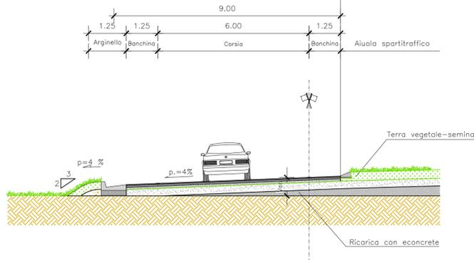
SEZIONE TIPO RAMI INGRESSO/USCITA ROTATORIA
