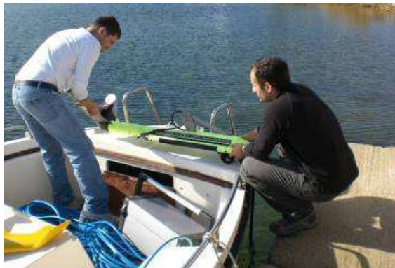
Figura 3-5 Side Scan Sonar Klein 3900.
