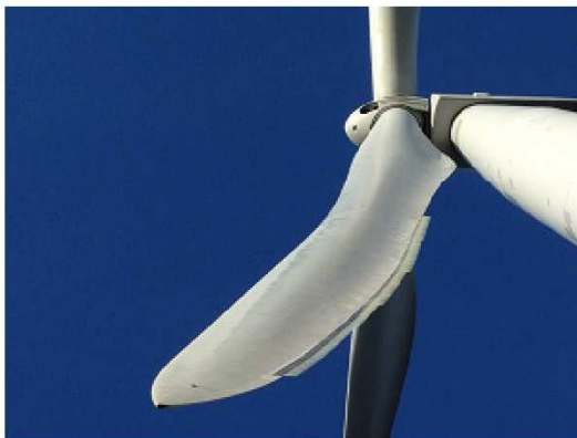
Fig. 1: LNTEs at the wind turbine rotor blade
