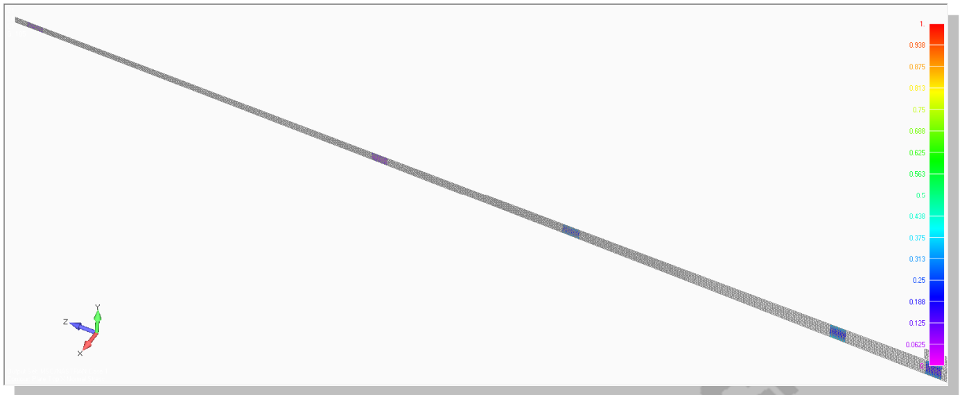
Figure 24 Leading edge shear web damage index, tip region
