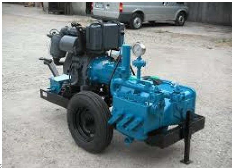
Figura 3: Pompa Triplex a piston.
