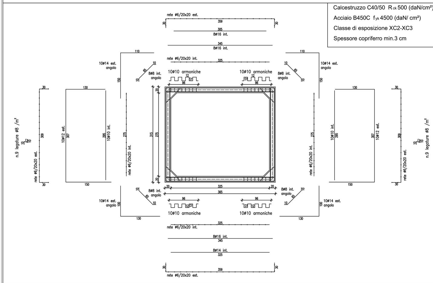
SCHEMA ARMATURE – SCATOLARE 300x175x200 sp.20cm
