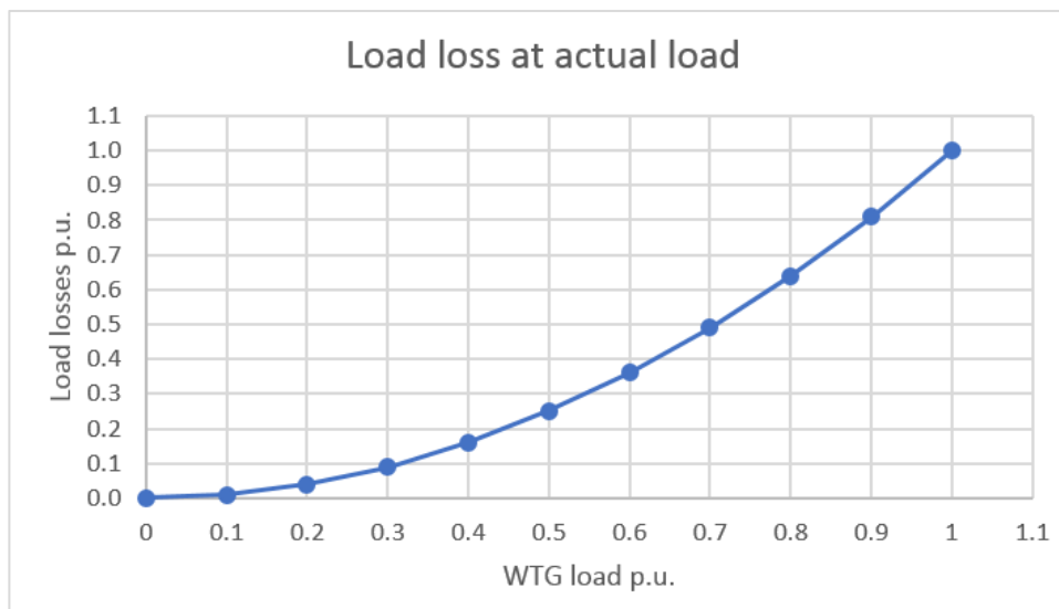
Figure 4-2- Transformer load losses scaling.
