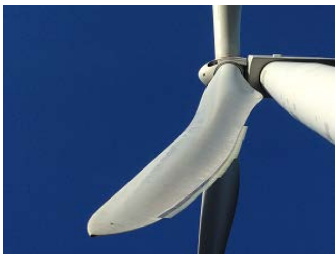
Fig. 1: LNTEs at the wind turbine rotor blade
