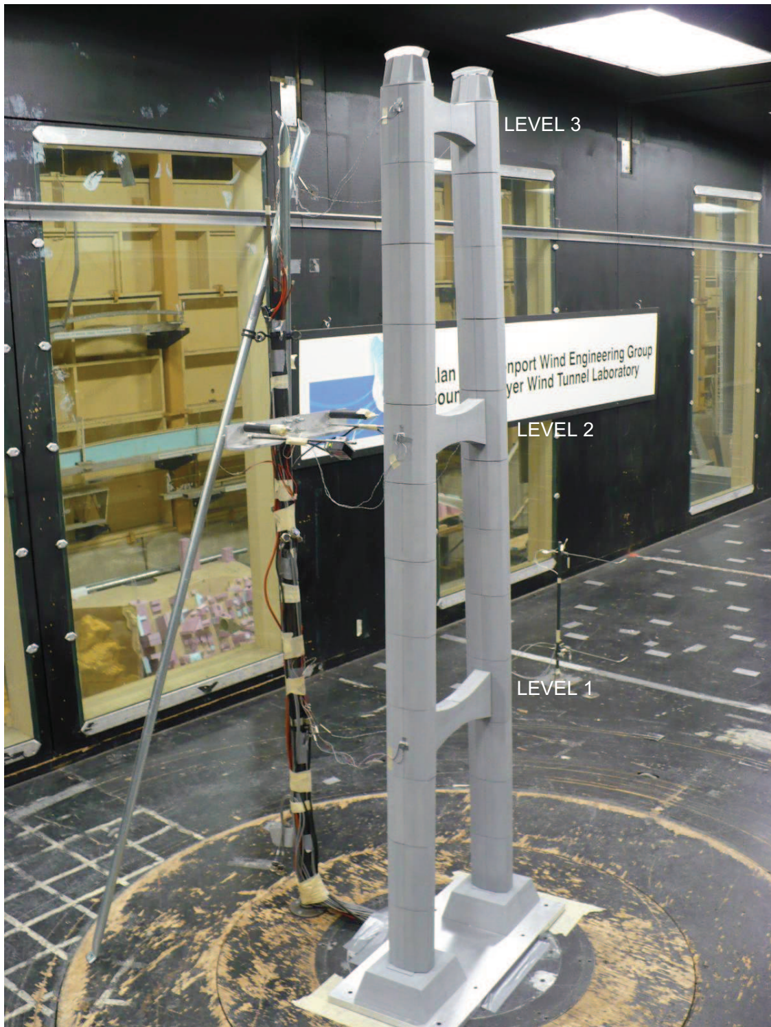
FIGURE 2.5 FROUDE SCALED AEROELASTIC MODEL, CONFIGURATION AND INSTRUMENTATION
