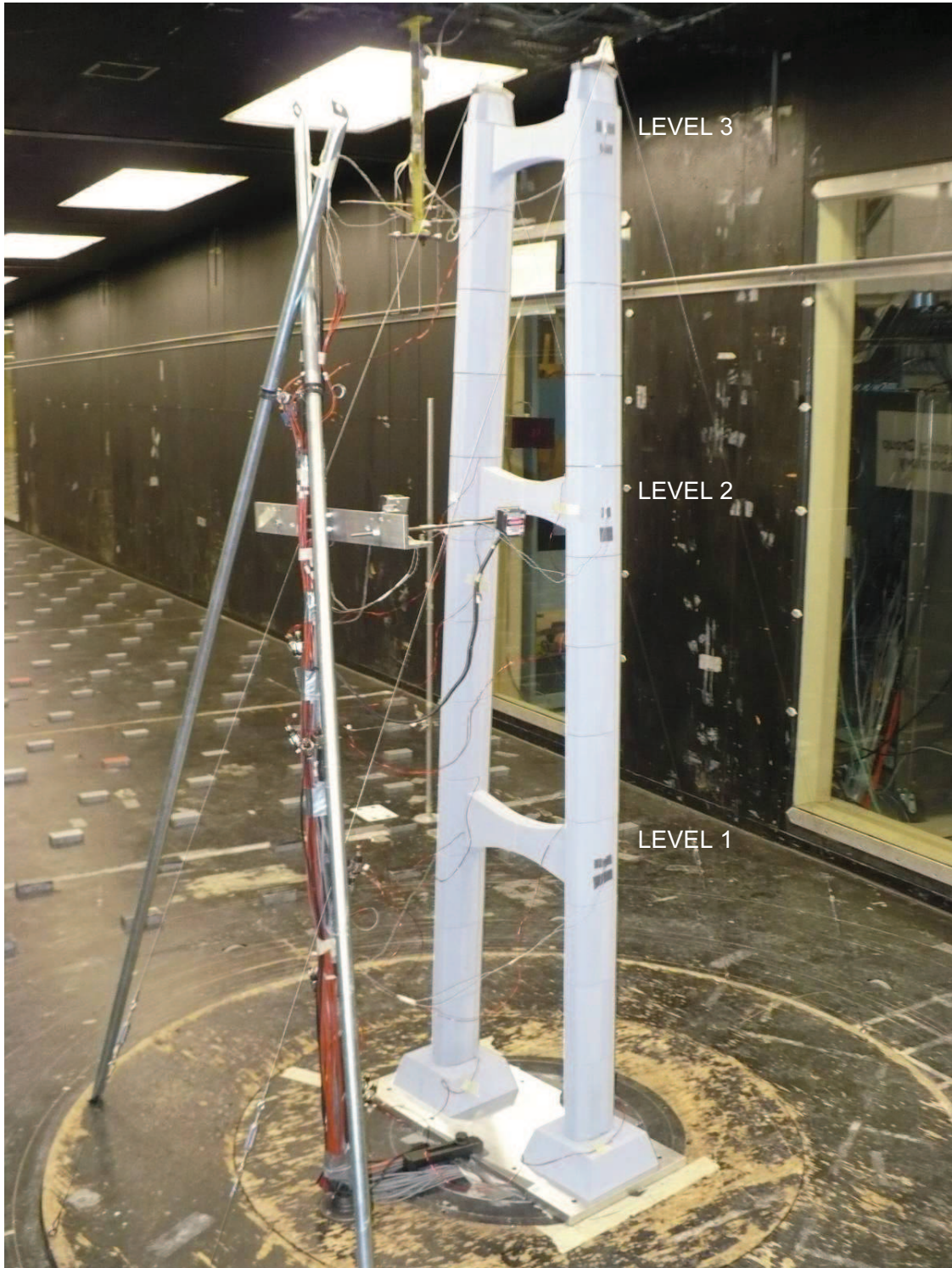
FIGURE 2.3 NON-FROUDE SCALED AEROELASTIC MODEL, CONFIGURATION AND INSTRUMENTATION
