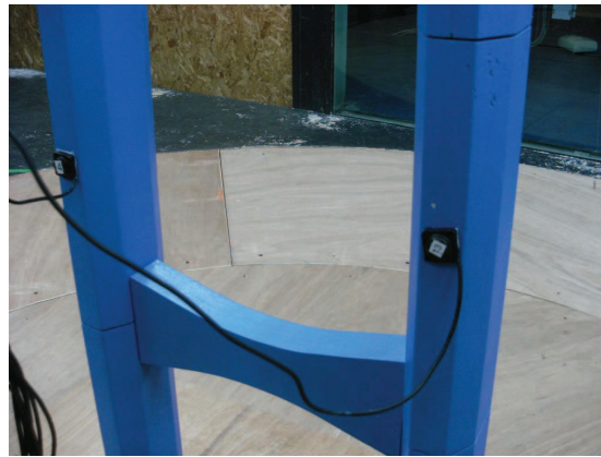
Fig C.1: Accelerometers, as mounted during testing
