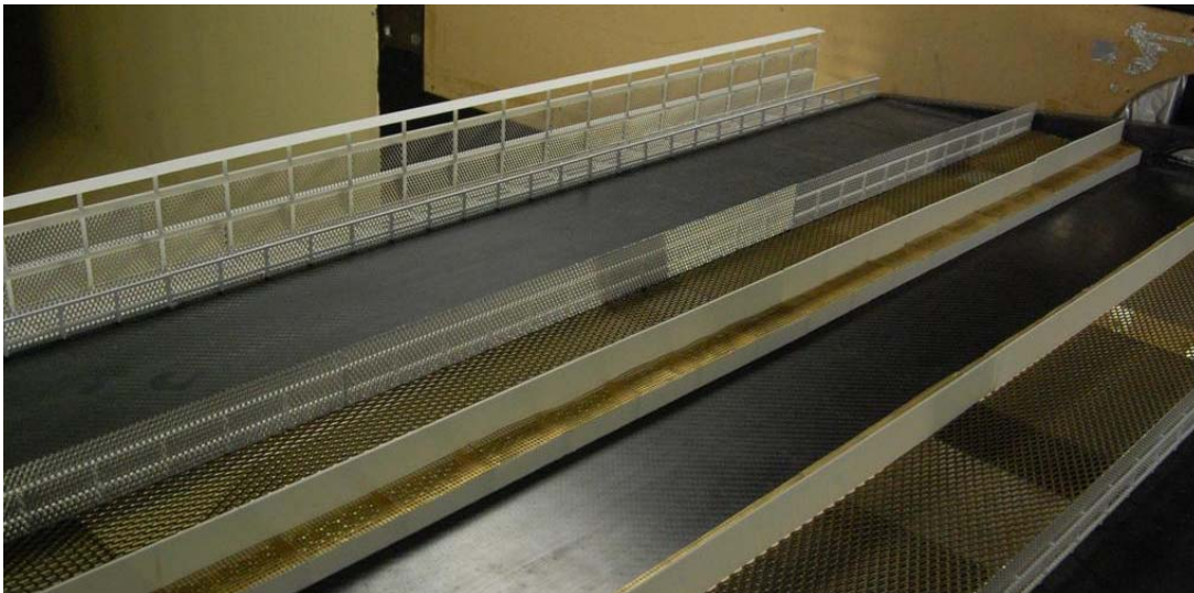
Figure 4.5 Deck section C5/63 with A screens and horizontal mesh between roadway and railway girders.
