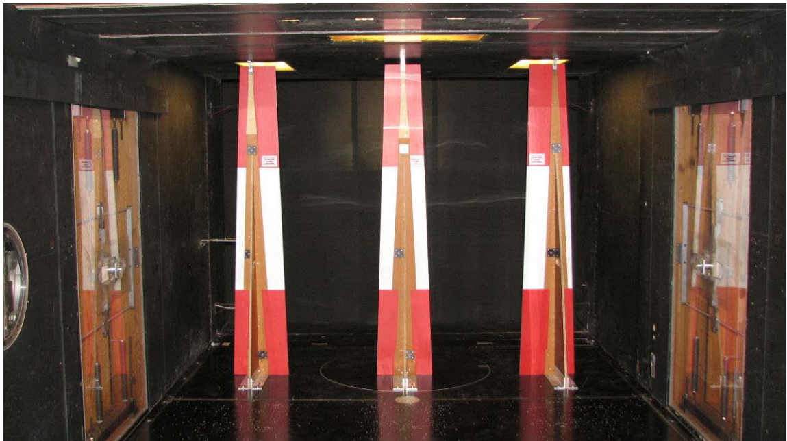
Figure 4.1. Turbulence generating spires in the wind tunnel up-wind of the model.
