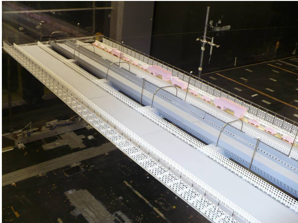
d) TRAFFIC Condition 2* – Road Traffic on Outward (Slow) Lane on Windward Girder, No Train Traffic
