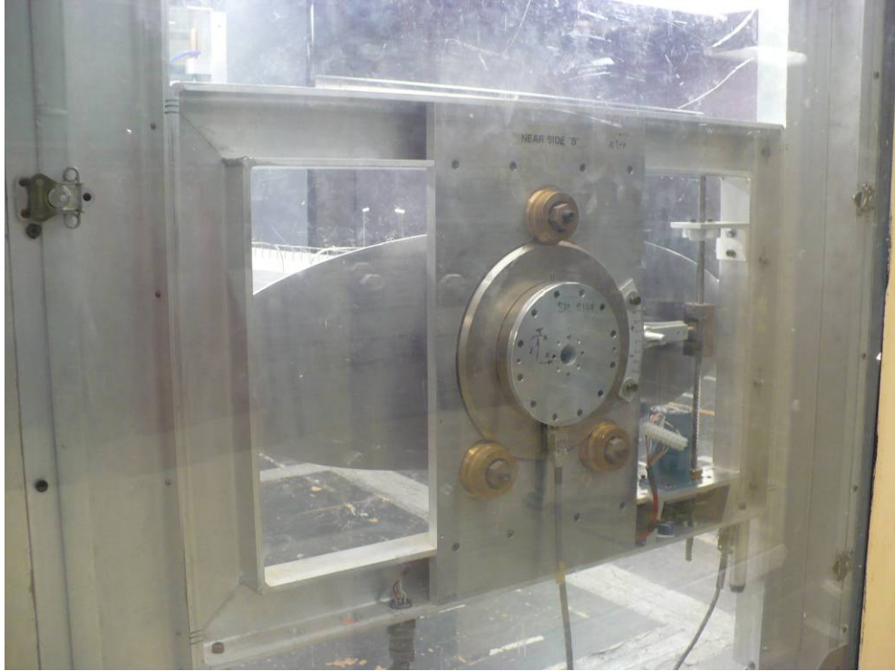
FIGURE 2.6 STATIC SECTION MODEL TEST RIG
