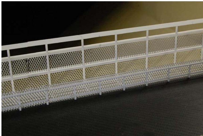
Figure B.2: Wind Tunnel Model – Close up View of the Wind Barriers (Screen A)
