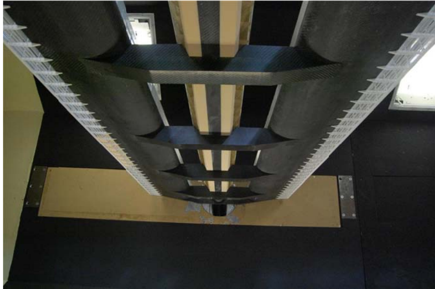
Figure B.4: Wind Tunnel Model - Close-Up View of Underside of Model with horizontal screens
