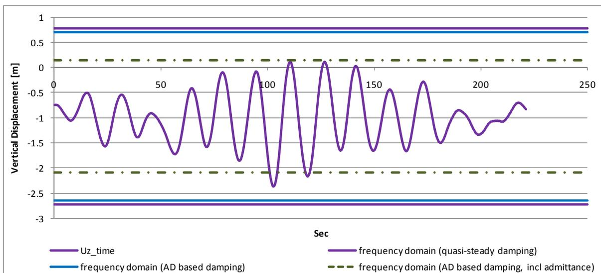
Figure 4.3 Comparison of vertical response  $U_z$  obtained from frequency domain and time domain buffeting analyses.
