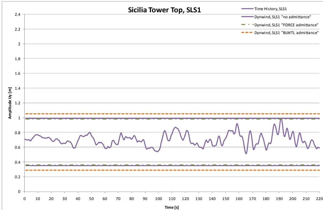
Figure 5.35 Buffeting comparisons along wind response, SLS1.
