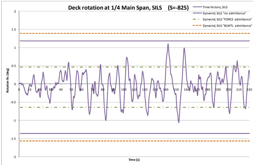
Figure 5.34 Buffeting comparisons torsion response, SILS.
