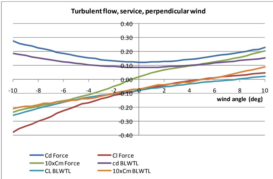
Figure 2.1 Static wind load coefficients from the two parallel tests (sub-tests D3 and D4), no traffic. Turbulent flow, perpendicular wind.
