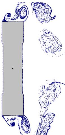
Figure 2.2 Cross beam cross section. Width = 4 m, Height = 17.74 m.
