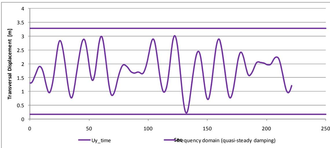
Figure 4.10 Comparison of transverse (along wind) response  $U_y$  obtained from frequency domain and time domain buffeting analyses.
