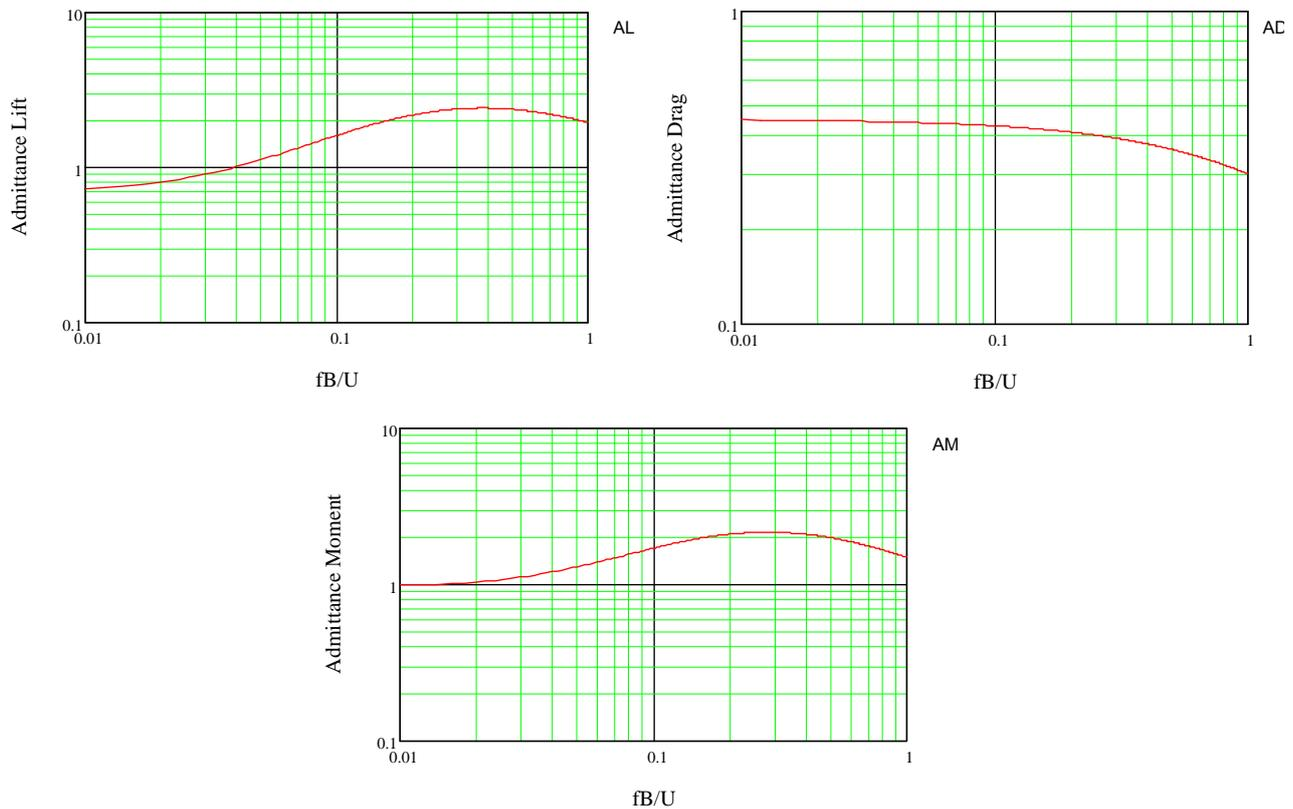
Figure 2.4 Aerodynamic admittances fitted to BLWTL measurements.
