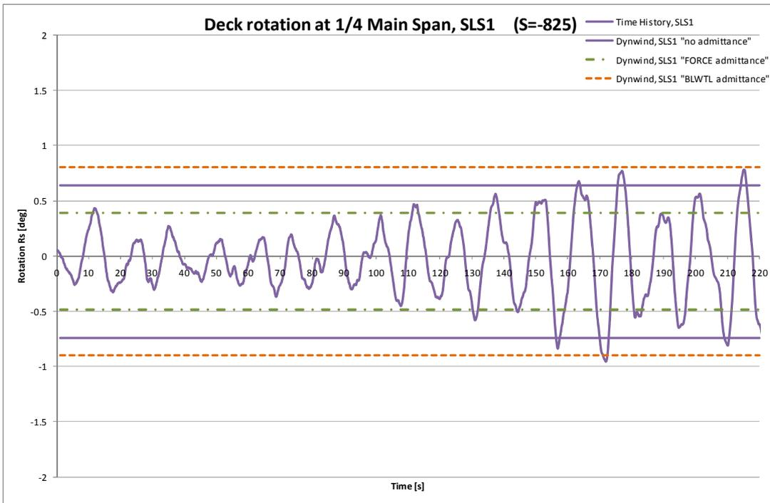
Figure 5.25 Buffeting comparisons torsion response, SLS1.
