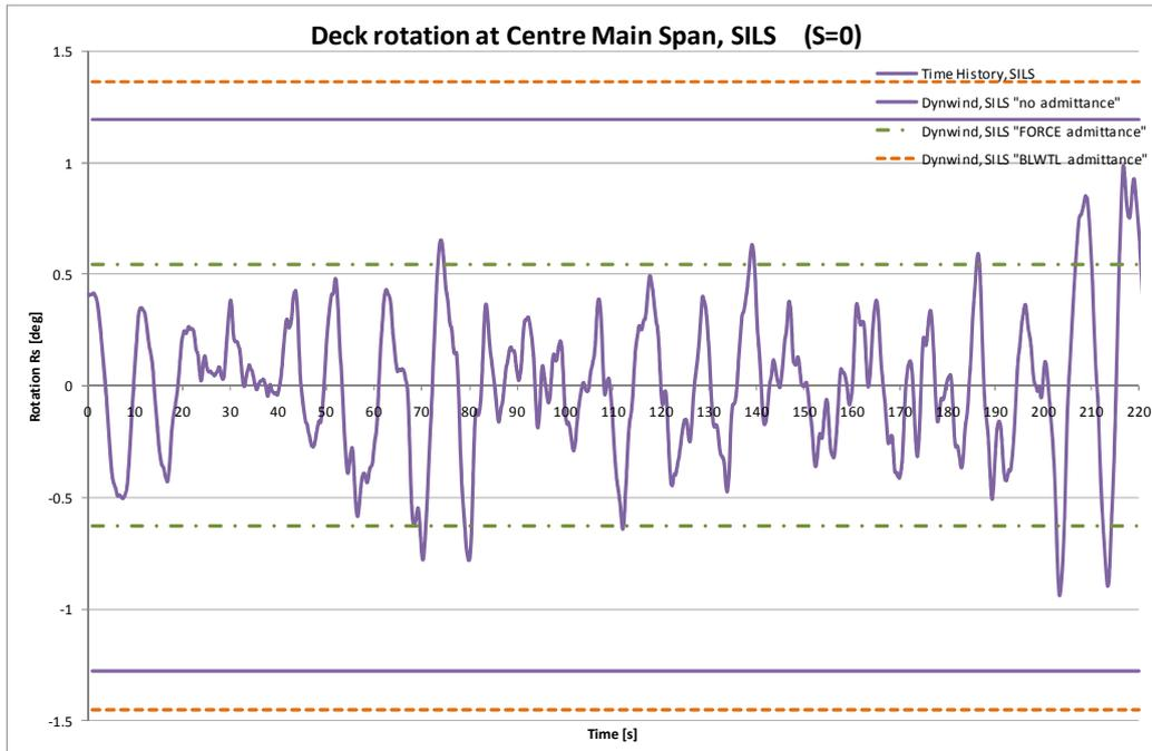
Figure 5.22 Buffeting comparisons torsion response, SILS.
