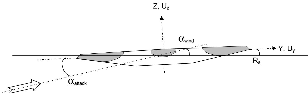
Figure 3.2 Definition of angle of attack of the wind assumed in the time history analyses.
