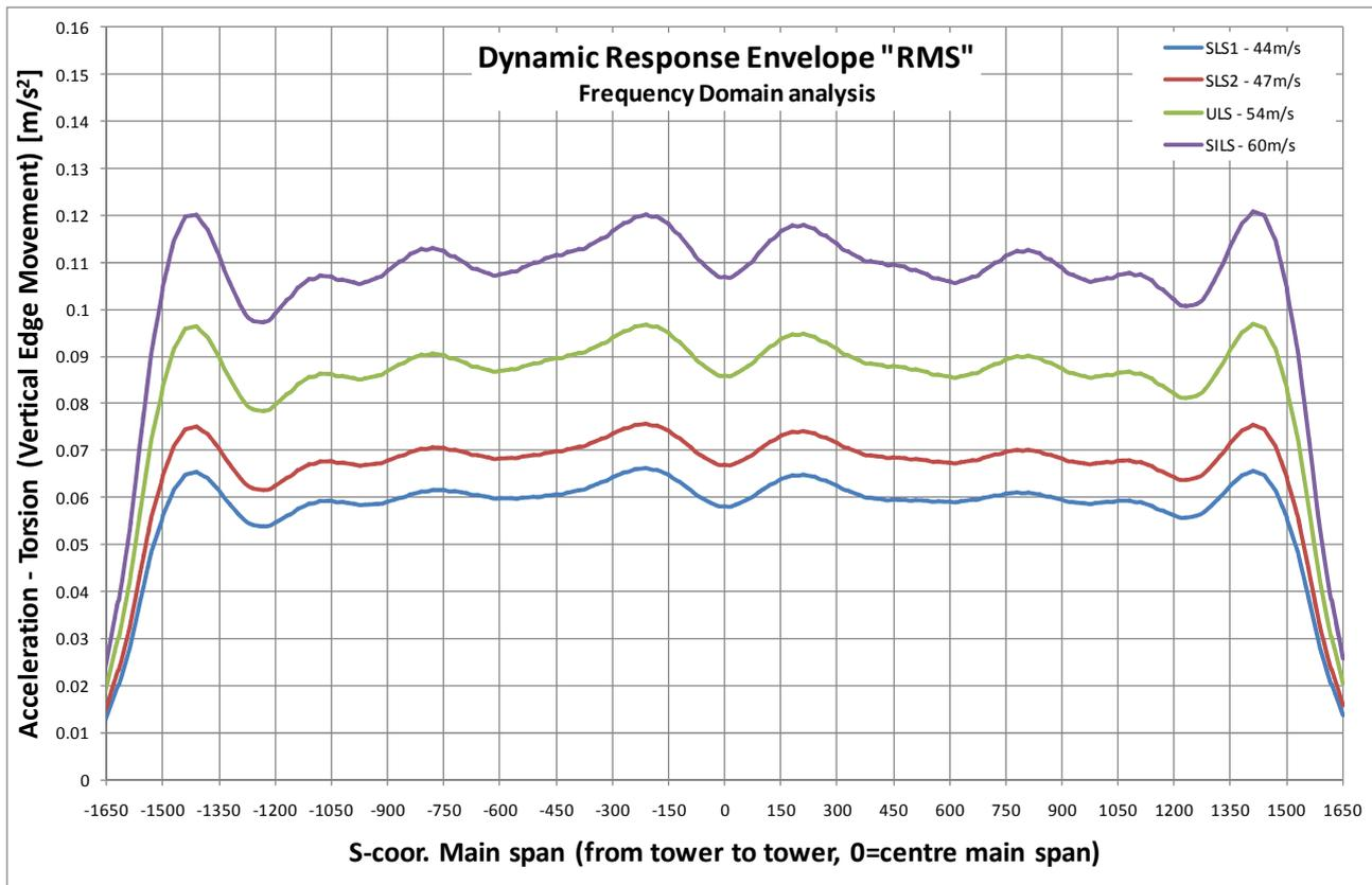
Figure 5.10 RMS vertical edge deflections along the span due to girder twist.
