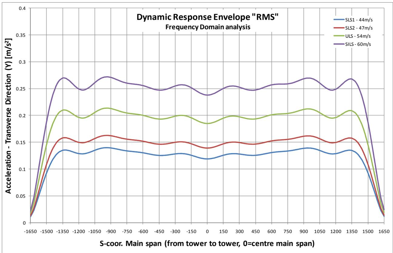
Figure 5.8 Horizontal RMS accelerations along span.
