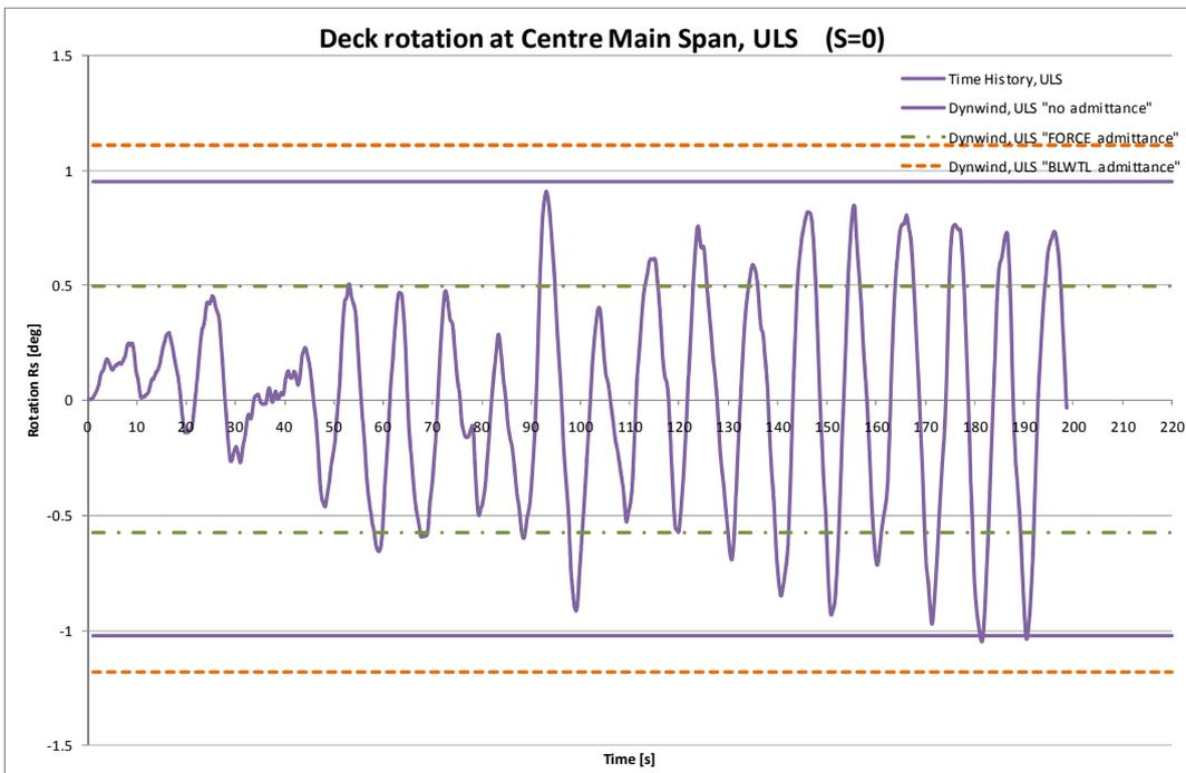
Figure 5.19 Buffeting comparisons torsion response, ULS.
