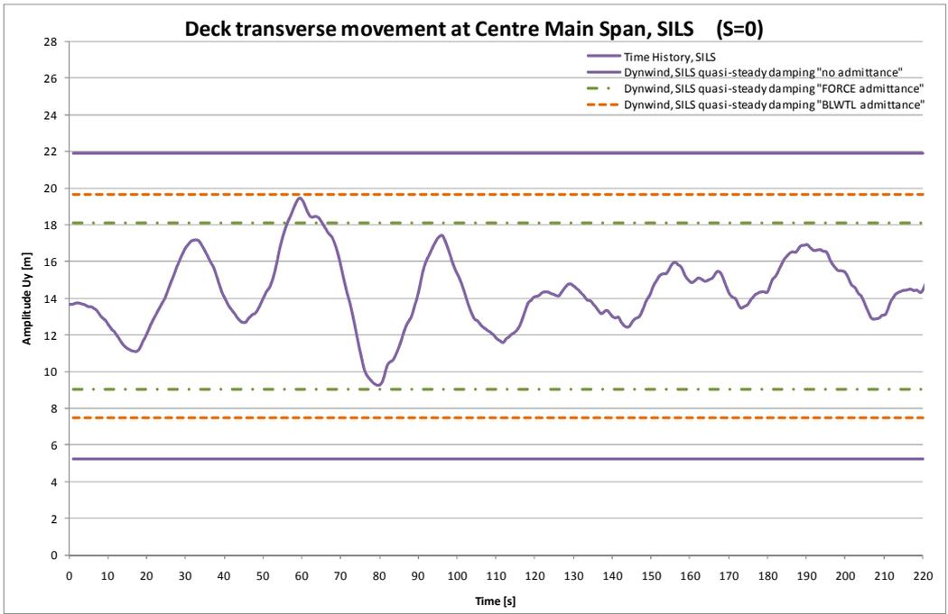
Figure 5.20 Buffeting comparisons orizontal response, SILS
