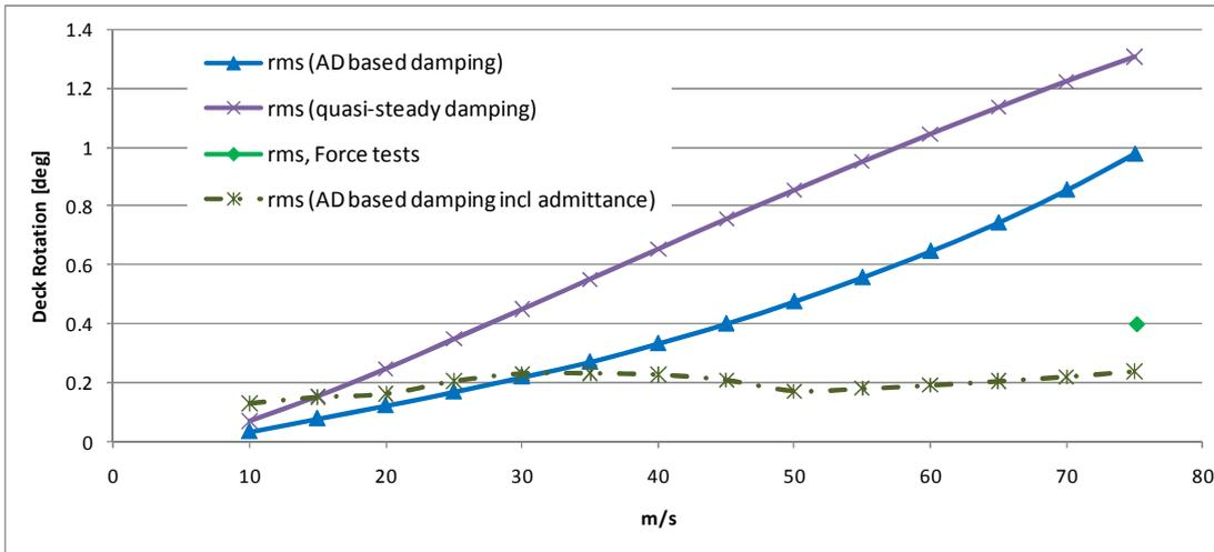
Figure 4.2 Torsion response  $R_s$  obtained from frequency domain buffeting calculations and wind tunnel tests at FORCE .
