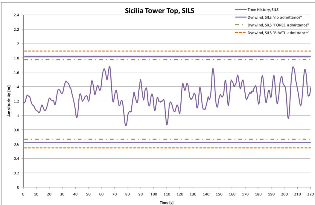
Figure 5.38 Buffeting comparisons along wind response, SILS.
