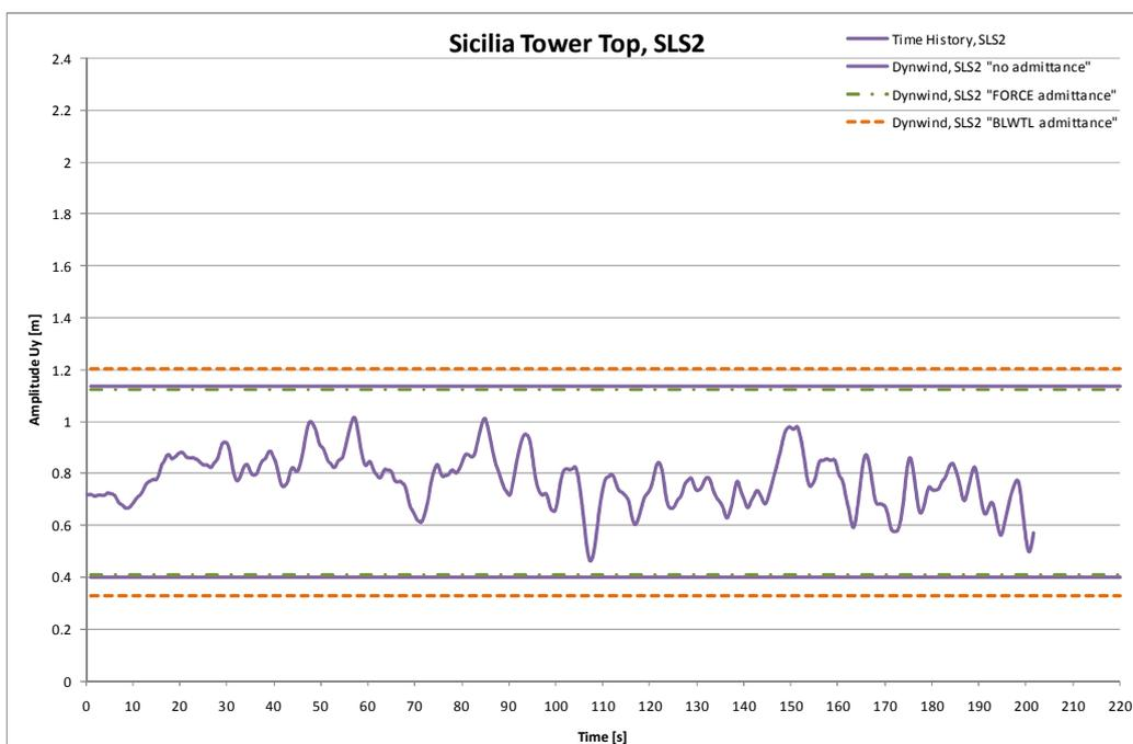
Figure 5.36 Buffeting comparisons along wind response, SLS2.
