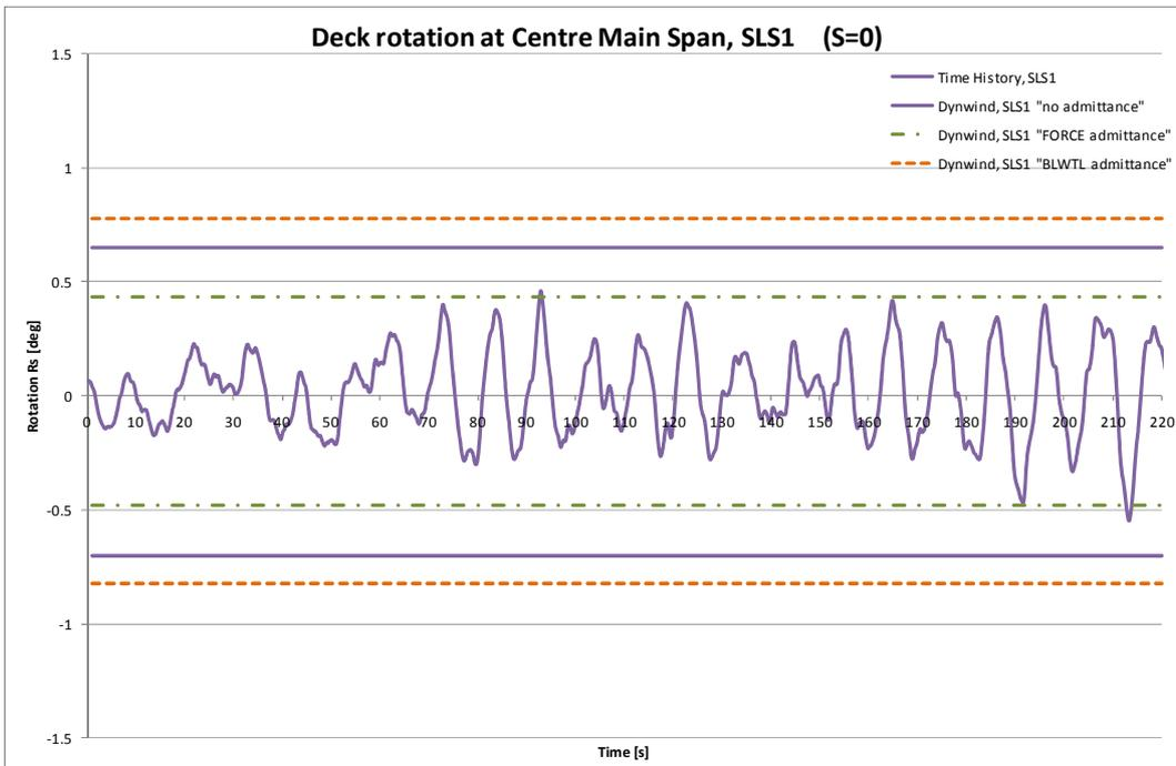
Figure 5.13 Buffeting comparisons torsion response, SLS1.
