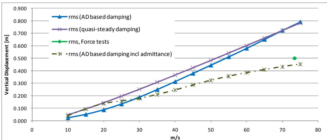
Figure 4.1 Vertical response  $U_z$  obtained from frequency domain buffeting calculations and wind tunnel tests at FORCE.
