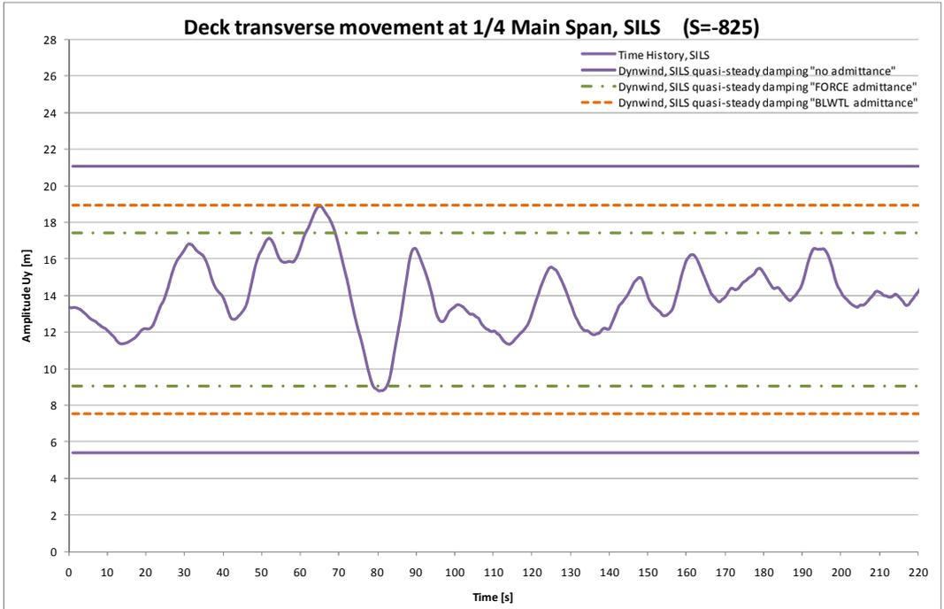
Figure 5.32 Buffeting comparisons horizontal response, SILS.
