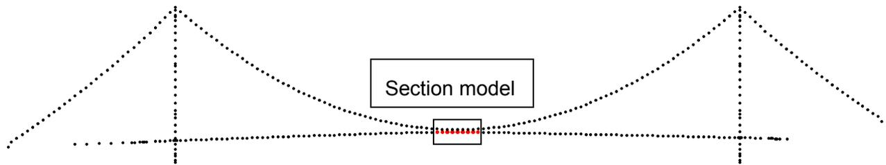
Figure 3.1 Overview of the nodes selected on the bridge for time series input.
