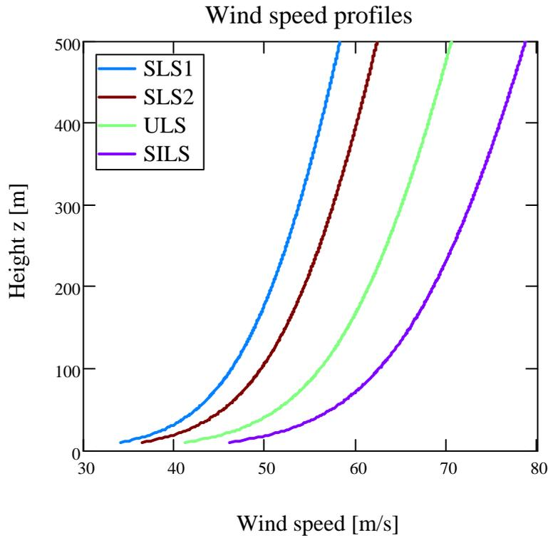
Figure 5.1 Mean wind speed as function of level above ground
