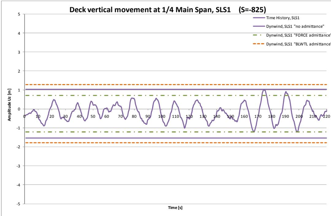
Figure 5.24 Buffeting comparisons vertical response, SLS1.
