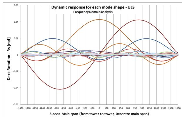
Figure 5.7 Vertical (lateral), vertical and torsion rms displacements and corresponding dominant modes in the buffeting analysis.
