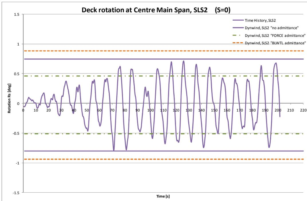
Figure 5.16 Buffeting comparisons torsion response, SLS2.
