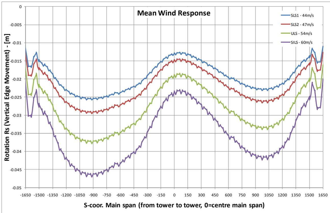
Figure 5.6 Angular displacement of the bridge girder for load conditions SLS1, SLS2, ULS and SILS.
