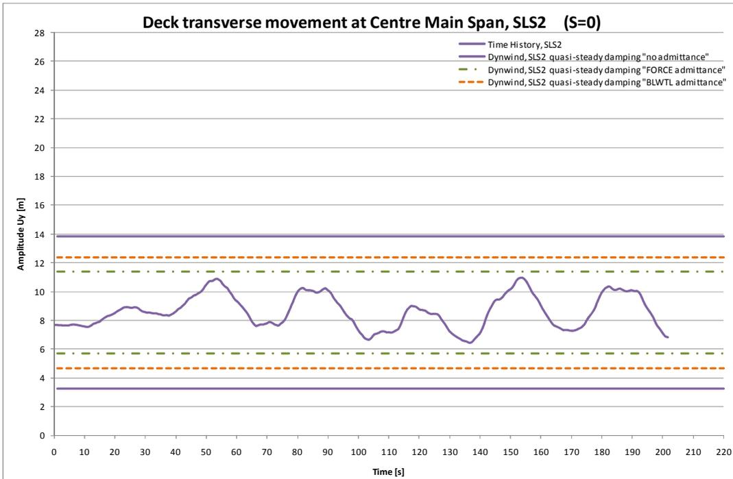
Figure 5.14 Buffeting comparisons horizontal response, SLS2.
