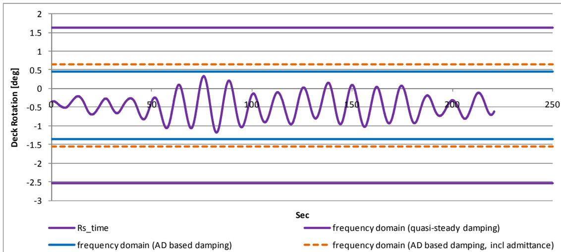
Figure 4.11 Comparison of torsion response  $R_s$  obtained from frequency domain and time domain buffeting analyses.
