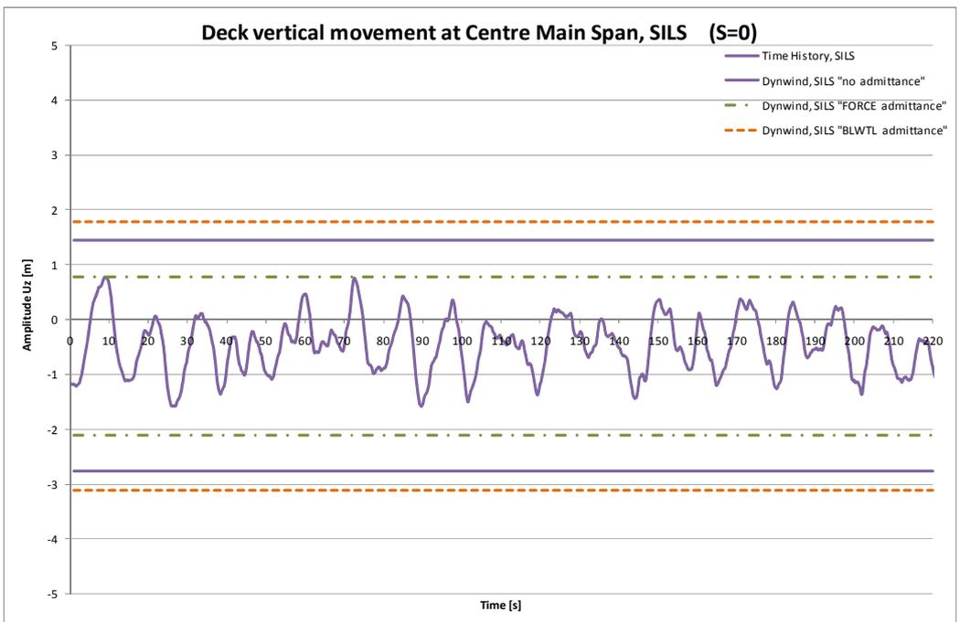
Figure 5.21 Buffeting comparisons vertical response, SILS.
