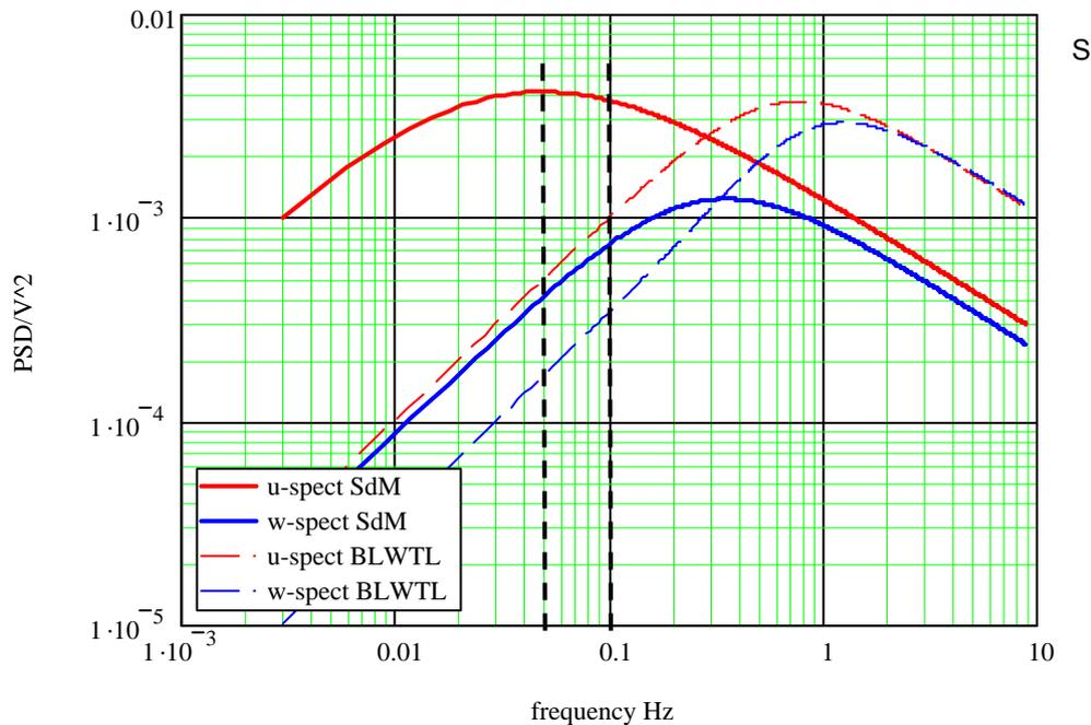
Figure 4.12 Power spectral distributions of longitudinal and vertical turbulence normalized by mean wind speed squared. SdM specification (thick solid lines), BLWTL (thin dashed lines).
