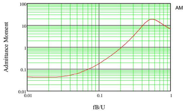
Figure 2.3 Aerodynamic admittances fitted to FORCE measurements.
