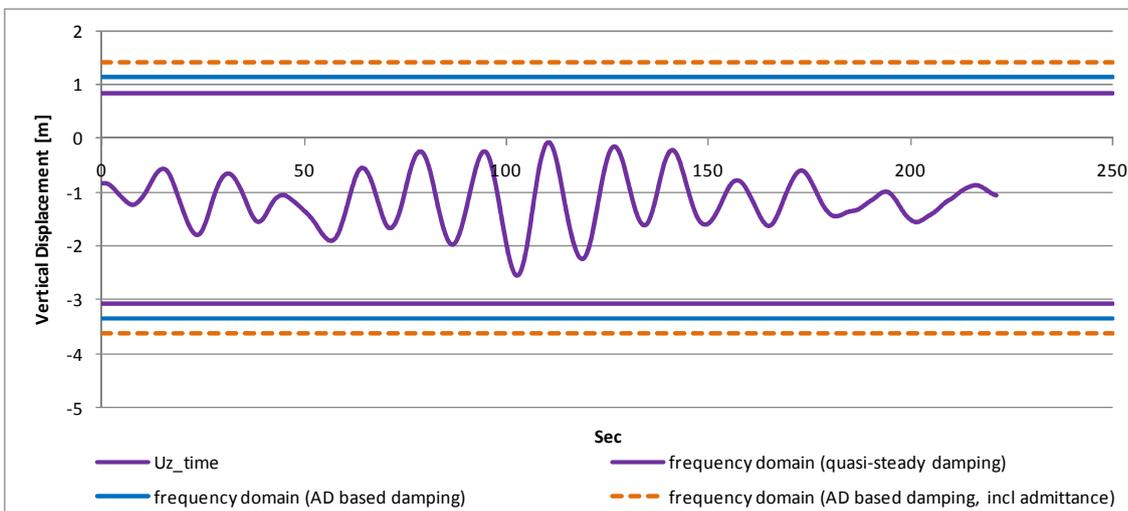
Figure 4.9 Comparison of vertical response  $U_z$  obtained from frequency domain and time domain buffeting analyses.
