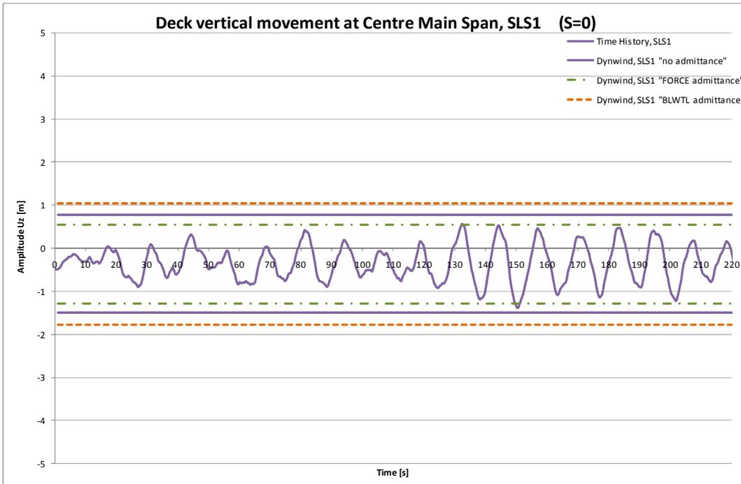
Figure 5.12 Buffeting comparisons vertical response, SLS1.
