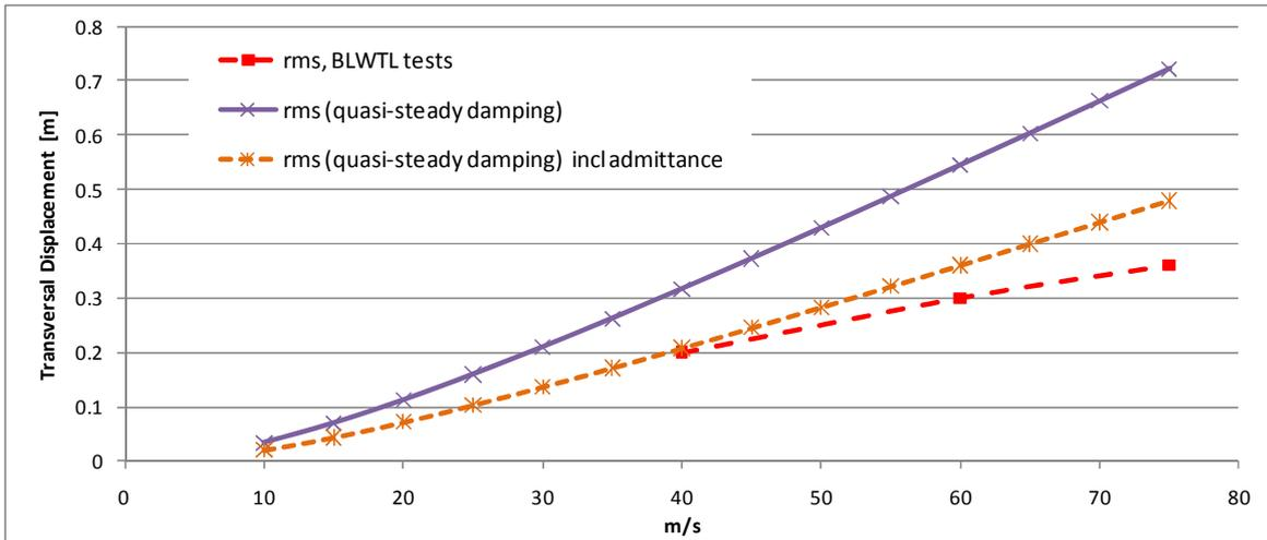
Figure 4.7 Transversal (along wind horizontal) response  $U_y$  obtained from frequency domain buffeting calculations and wind tunnel tests at BLWTL.
