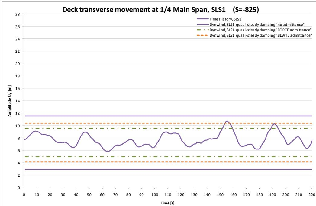
Figure 5.23 Buffeting comparisons horizontal response, SLS1.
