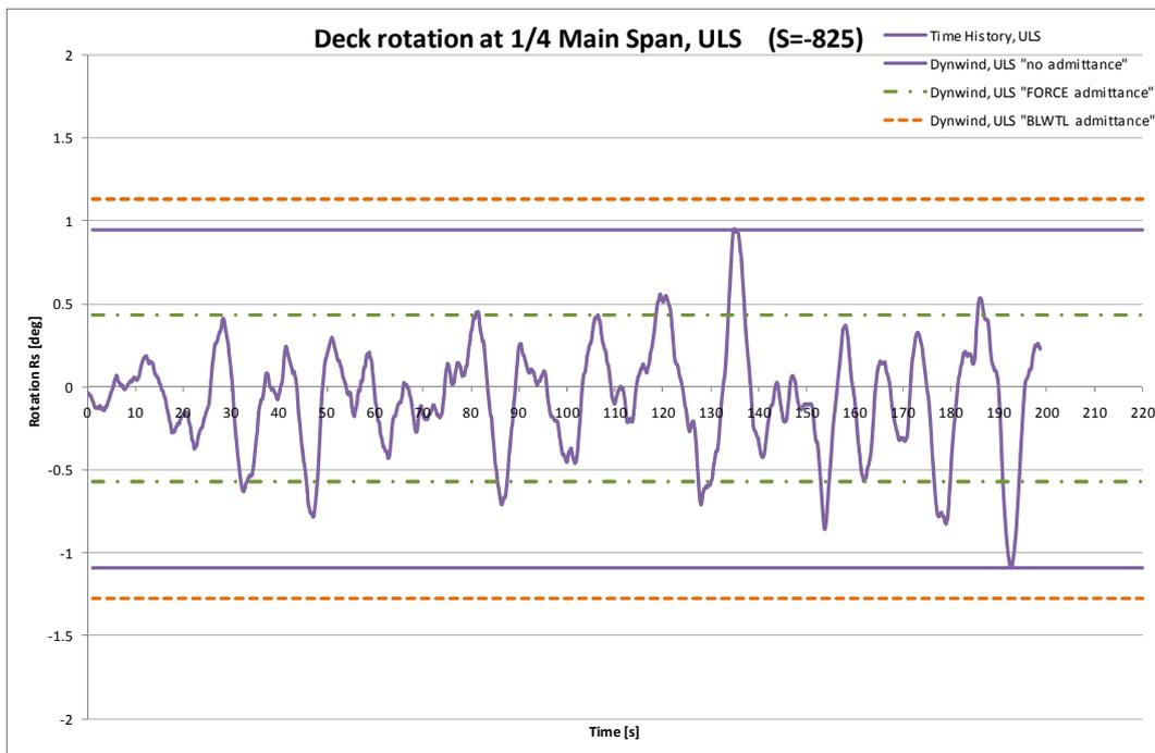
Figure 5.31 Buffeting comparisons torsion response, ULS.
