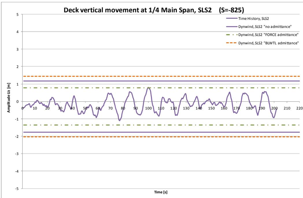
Figure 5.27 Buffeting comparisons vertical response, SLS2.
