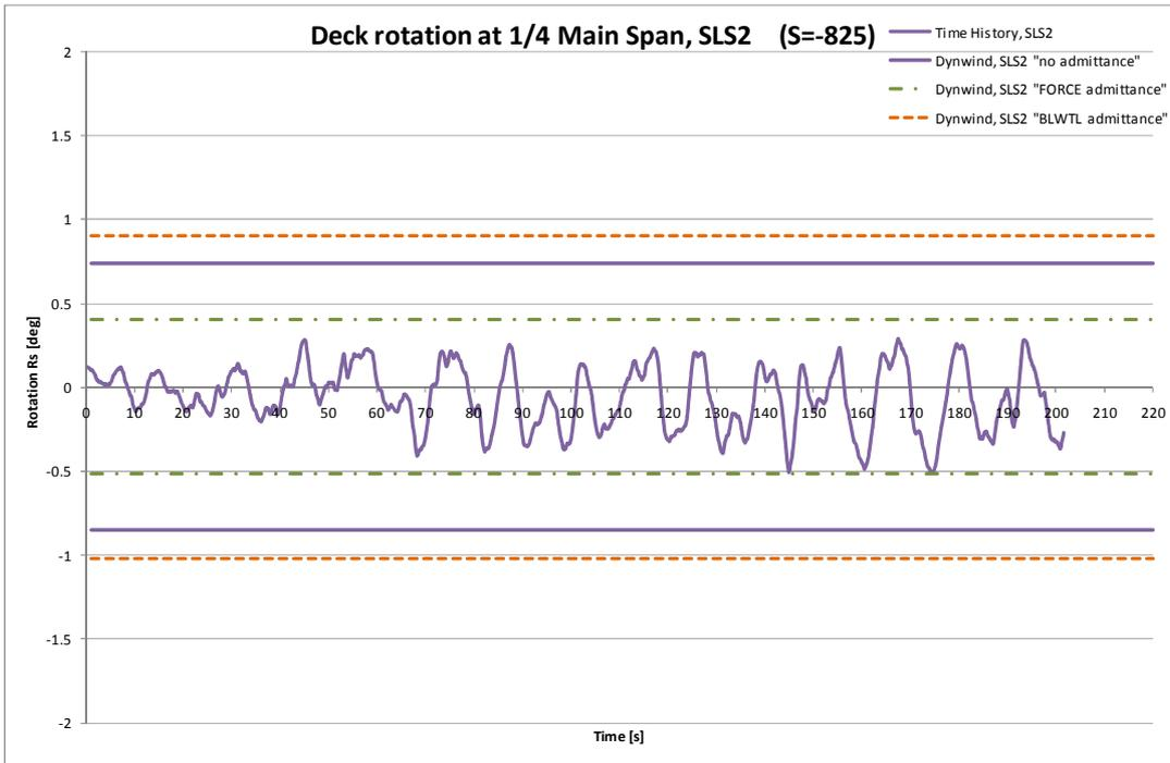
Figure 5.28 Buffeting comparisons torsion response, SLS2.
