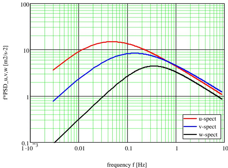
Figure 5.3 Turbulence spectra for the SILS condition specified by SdM
