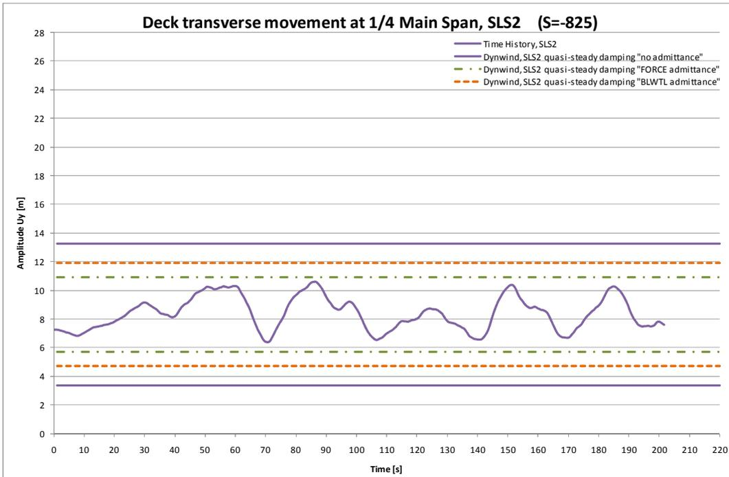
Figure 5.26 Buffeting comparisons horizontal response, SLS2.
