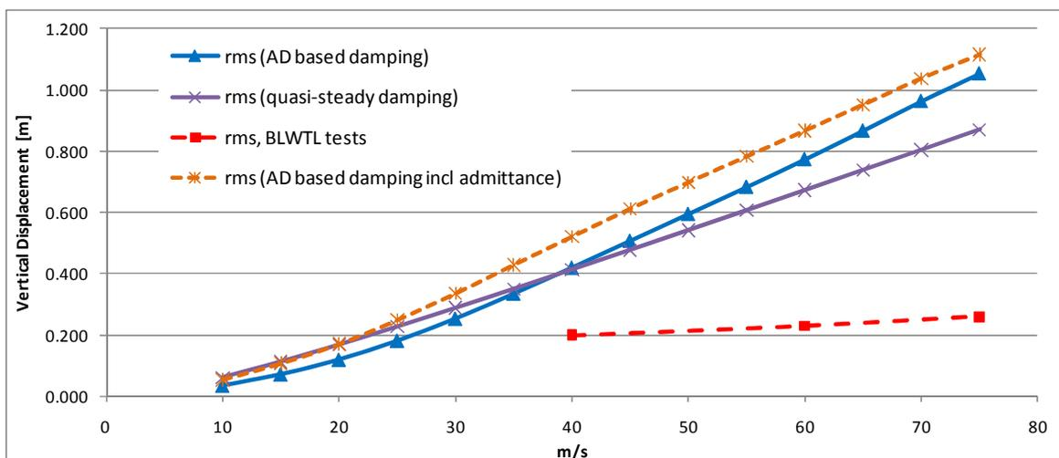
Figure 4.6 Vertical response  $U_z$  obtained from frequency domain buffeting calculations and wind tunnel tests at BLWTL.
