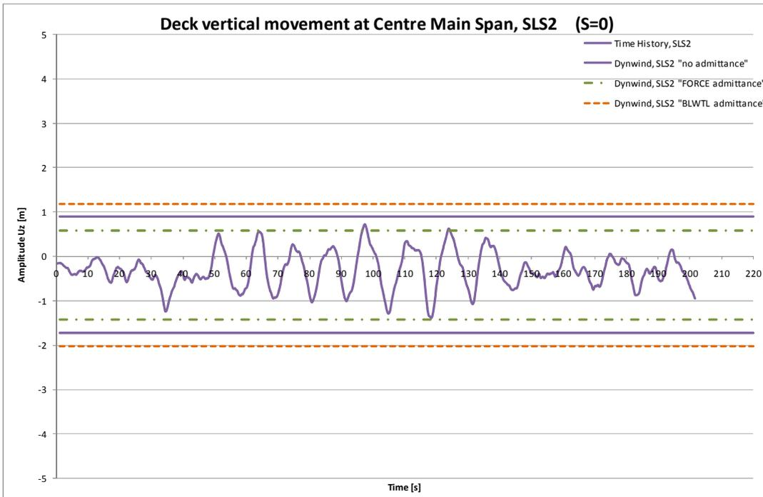
Figure 5.15 Buffeting comparisons vertical response, SLS2.
