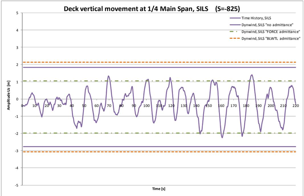
Figure 5.33 Buffeting comparisons vertical response, SILS.
