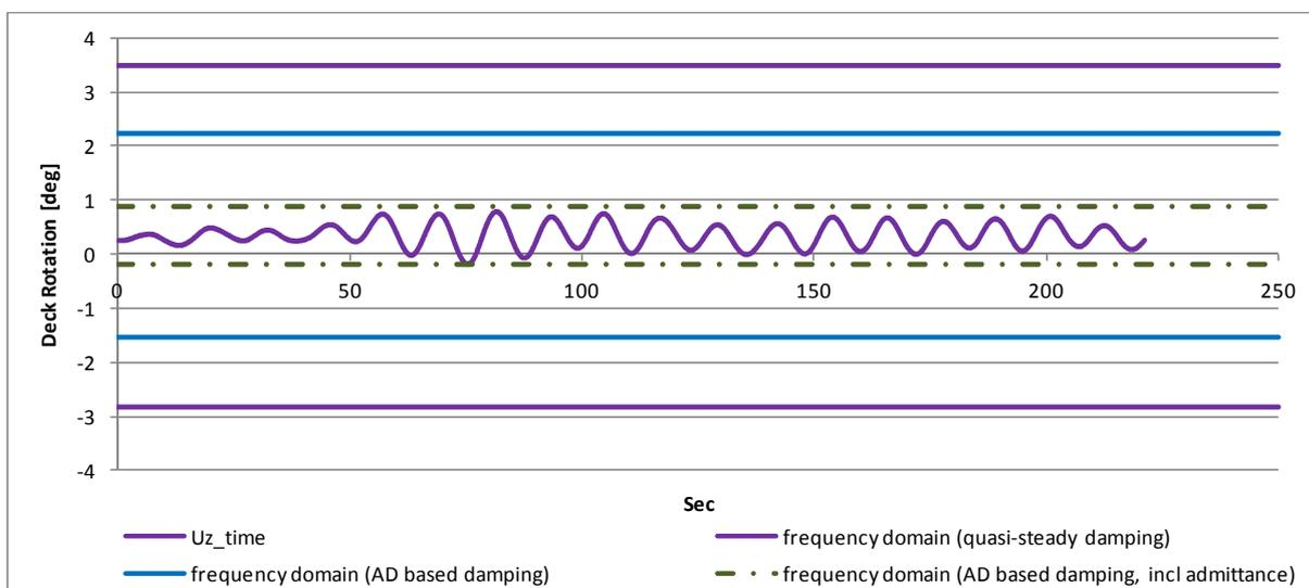
Figure 4.4 Comparison of torsion response  $R_s$  obtained from frequency domain and time domain buffeting analyses.
