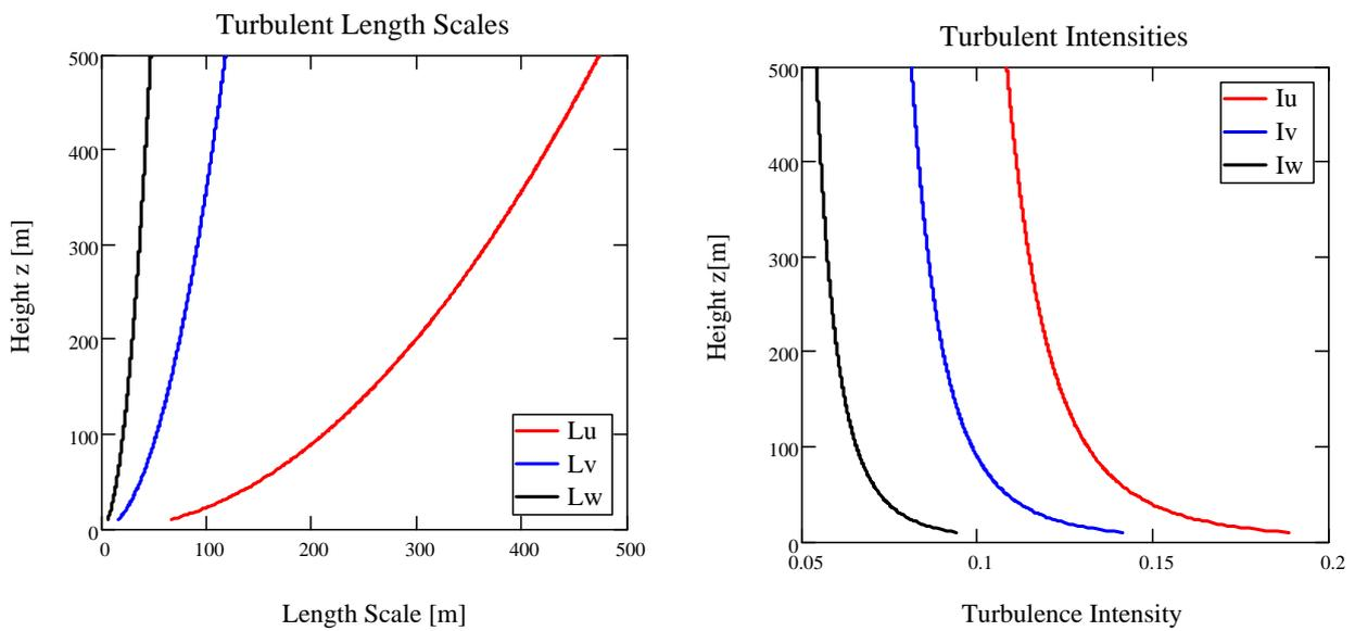
Figure 5.2 Length scales and turbulence intensities specified by SdM
