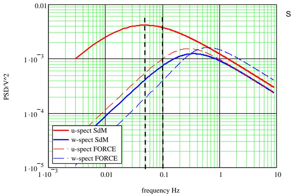
Figure 4.5 Power spectral distributions of longitudinal and vertical turbulence normalized by mean wind speed squared. SdM specification (thick solid lines), FORCE (thin dashed lines).
