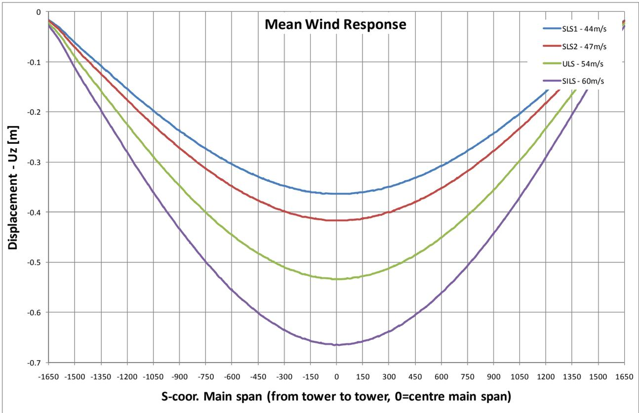
Figure 5.5 Vertical displacement of the bridge girder for load conditions SLS1, SLS2, ULS and SILS.
