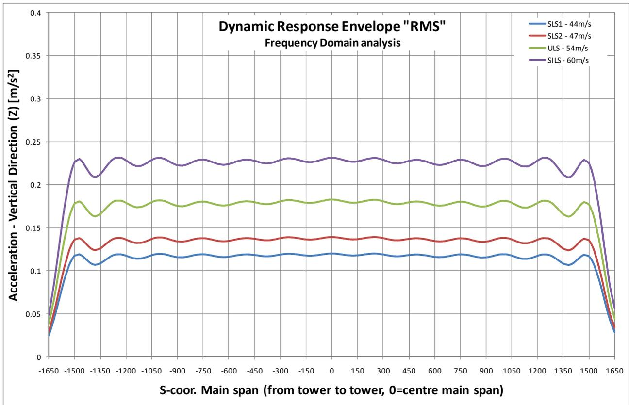
Figure 5.9 Vertical RMS accelerations along the span at the centre line of the railway girder.
