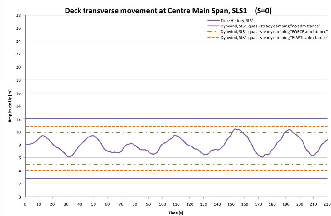
Figure 5.11 Buffeting comparisons horizontal response, SLS1.
