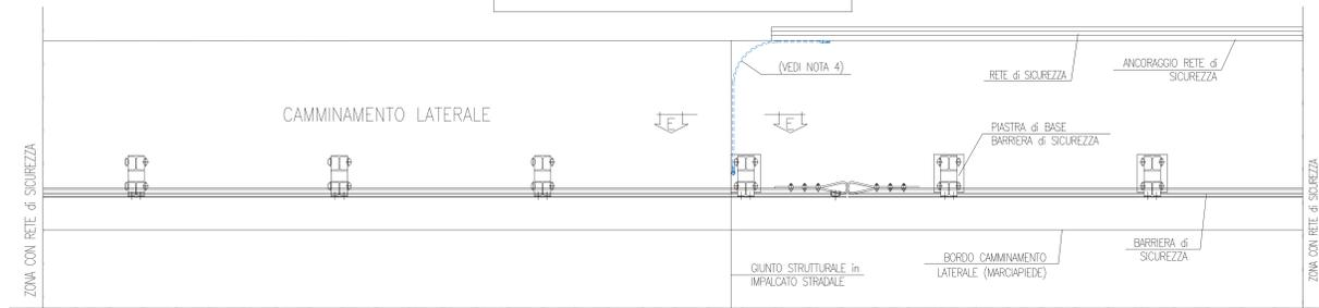
(NOTA 4): IN CORRISPONDENZA DELLA FINE DELLA RETE ELETTROSALDATA E' PREVISTO IL COLLEGAMENTO TRA STRUTTURA PER RETE e BARRIERA di SICUREZZA, MEDIANTE COLLEGAMENTO IN CORDA d'ACCIAIO ZINCATO 50mm<sup>2</sup> CON TERMINALI AD OCHHELLO Ø IN RAME 35mm<sup>2</sup> CON CAPICORDA IN RAME STAGNATO
