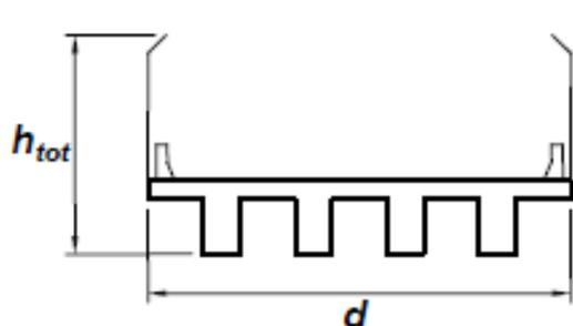
$$c_{fx} = \begin{cases} \frac{1,85}{d/h_{tot}} - 0,10 & 2 \leq d/h_{tot} \leq 5 \\ \frac{1,35}{d/h_{tot}} & d/h_{tot} > 5 \end{cases} \quad (G.24a)$$
