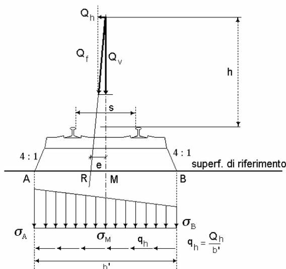
$$L_{trasm} = 1.5 + [H_{p-R,sup}/4 + S_s/2] * 2 = 3.30 \text{ m}$$
