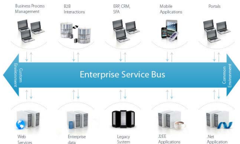
Figure 3.2.1 Basic communication concept of ESB (source: http://integrella.com )
