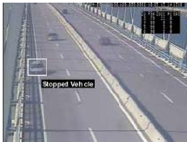
Figure 6.2: Example showing an AID system detecting a stopped vehicle on a bridge
