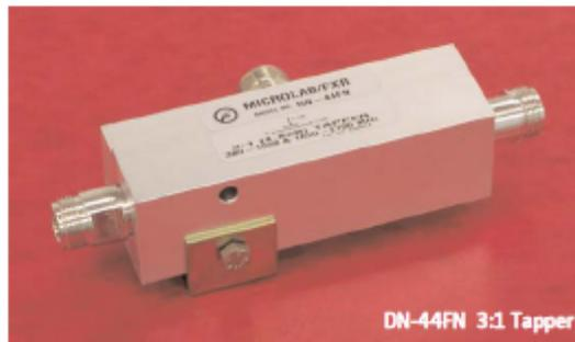
Microlab DN-x4FN series of Tappers unevenly split high power cellular signals in fixed ratios from 1000:1 to 2:1 with minimal reflections or loss over the wireless bands in the range 350 - 2,700 MHz, (there is no coupling 1550 to 1650 MHz). The innovative asymmetric design ensures an excellent Input VSWR and coupling flatness across the band, even down to a 2:1 split. If DC Continuity/AISG to the branch line is a requirement, see the DK-x4FN series.
