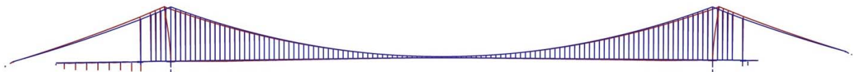
Figure 5.1: Reference condition (red line is deformed state at scale25) - it is important to notice that there is almost no displacements of neither deck nor towers visible, even when multiplying all displacement by a factor of 25.
