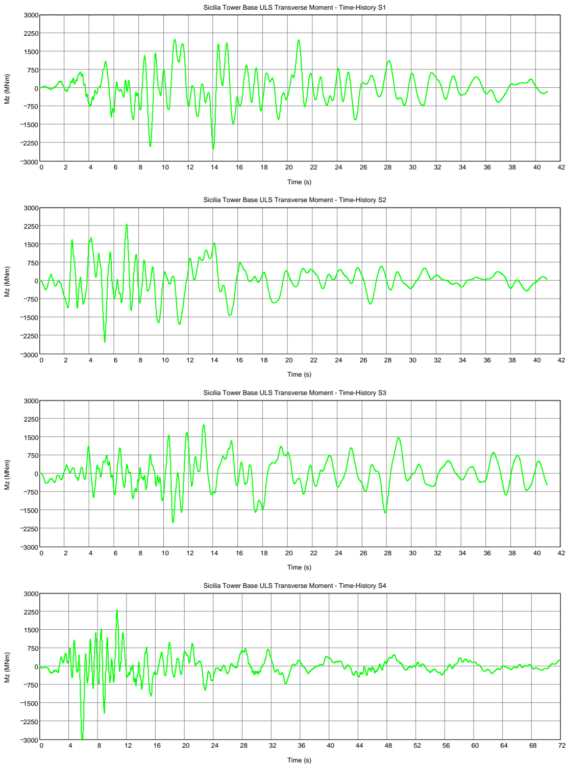
Figure A-17: Sicilia tower base ULS seismic transverse moments as a function of time for Sicilia time-history inputs 1 to 4.
