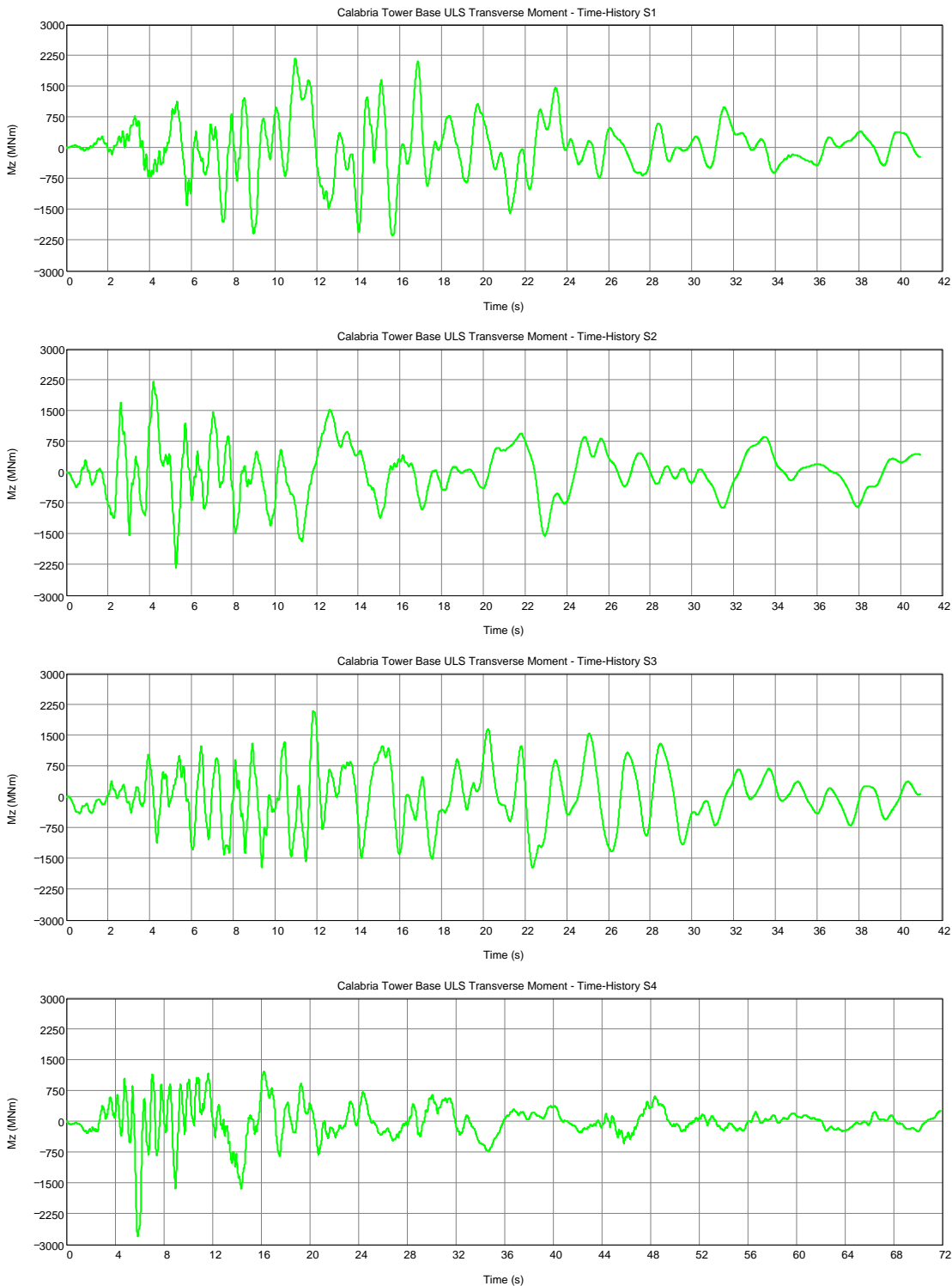
Figure A-29: Calabria tower base ULS seismic transverse moments as a function of time for Sicilia time-history inputs 1 to 4.
