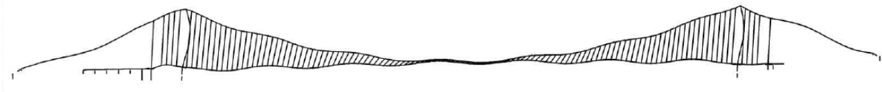
Figure 7-1: Mode 101 - Period 2.49 s - Frequency 0.40 Hz.
