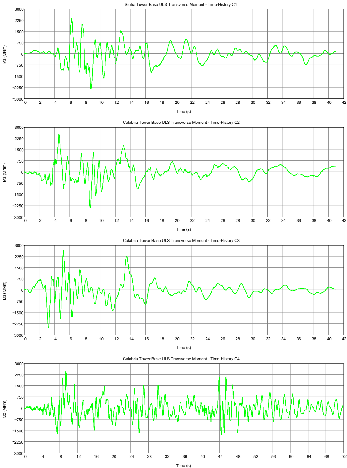
Figure A-30: Calabria tower base ULS seismic transverse moments as a function of time for Calabria time-history inputs 1 to 4.
