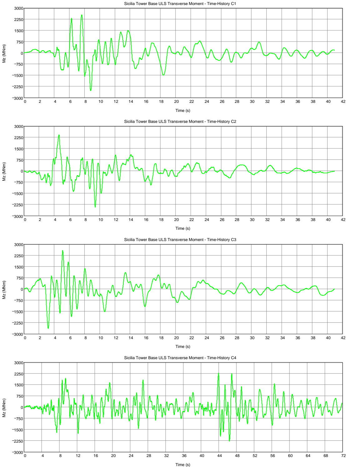
Figure A-18: Sicilia tower base ULS seismic transverse moments as a function of time for Calabria time-history inputs 1 to 4.
